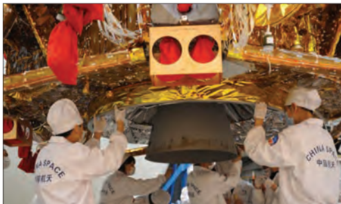
The underside of the lander has a nozzle for a large, new throttleable rocket engine and landing gear similar to Apollo lunar modules. The Chinese lander scales to about 40% of an Apollo descent stage and appears to be a formal prototype for eventual scale-up to a manned configuration. Credit: China Space News/NASASpaceflight.com/Planetary Society.
