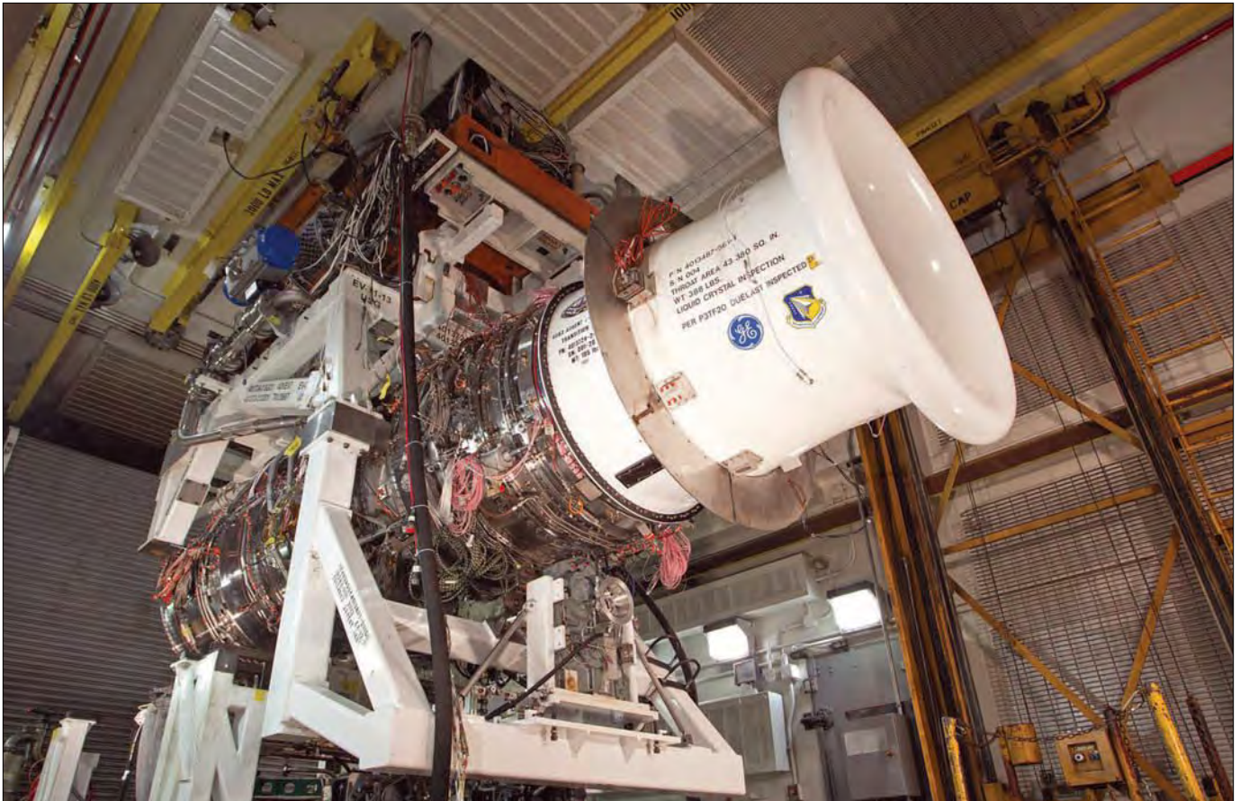
General Electric's Adaptive Versatile Engine Technology demonstrator, or Advent, achieved the highest temperature ever recorded inside a jet engine, the company reported in 2014. Advent tested heat-resistant ceramic-matrix composites. The white object on the right side, called a bell mouth, directed air into the engine, that has since been disassembled.
