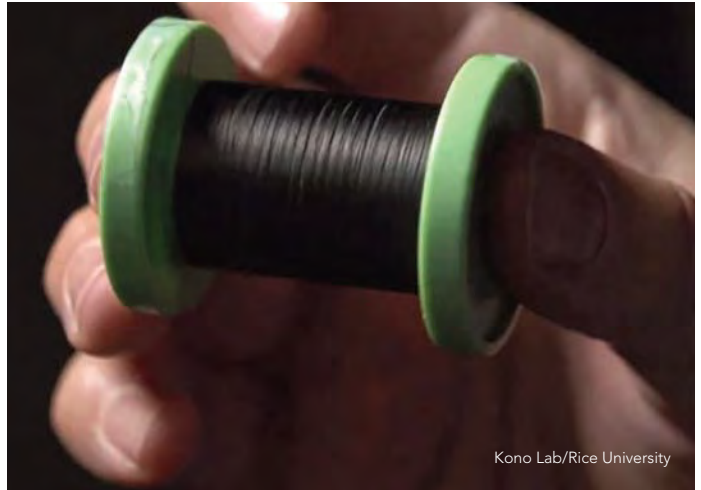
A spool of pure carbon nanotube fibers. Combining nanotubes with copper could transmit much more current while reducing weight of power cables.
