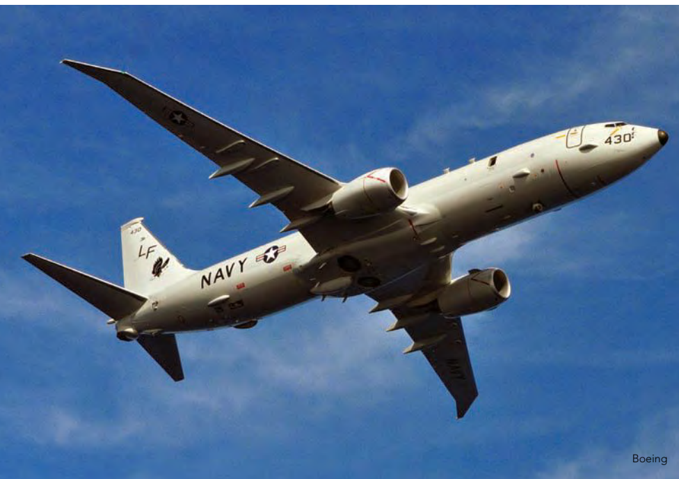
Boeing used the 737-800 as the foundation for the U.S. Navy's P-8 Poseidon. So far, India is the only other customer for the maritime surveillance aircraft.
