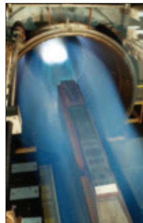
In 2008 the SJX61 successfully completed ground tests simulating Mach-5 flight conditions at NASA Langley.
