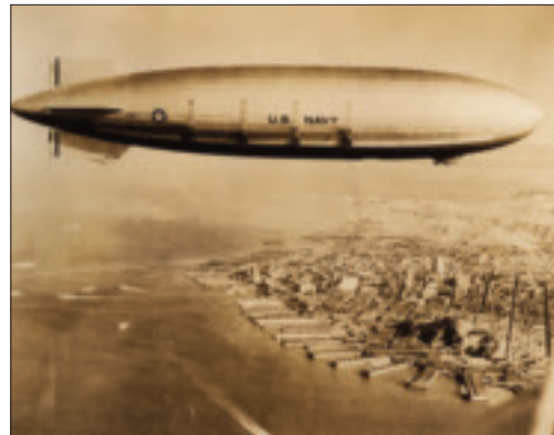
The USS Macon was a familiar sight across the U.S. The Macon was constructed with a built-in aircraft hangar and a trapeze launch and recovery system to facilitate fighter planes intended to protect the aircraft in war.
