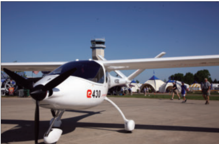
Power for the E430 comes from up to five battery packs.
