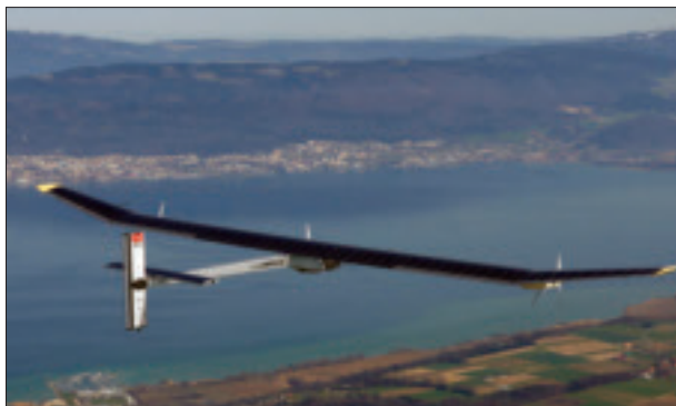
The Solar Impulse uses more than 11,000 solar cells to charge its batteries.
