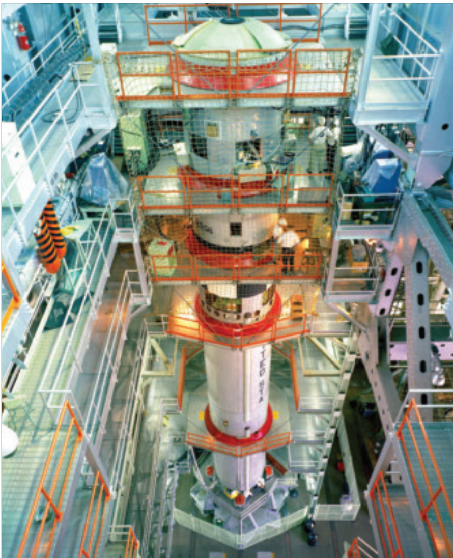
Martin's Baltimore plant in Middle River, Maryland, conducted assembly and checkout of the Titan IIs selected for Gemini. Gemini-Titan GT-2 (the second unmanned Gemini launch) stands in the test cell in D building in 1964. It flew on January 19, 1965. Courtesy: Glenn L. Martin Maryland Aviation Museum.
