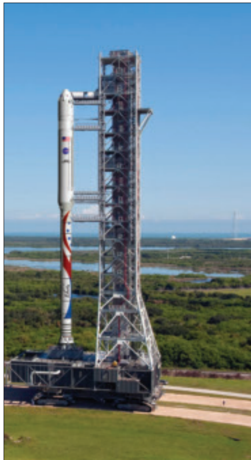
The first stage of ATK's two-stage Liberty is derived from the shuttle program; the second stage has achieved 46 consecutive launches as the core of the Ariane V.
