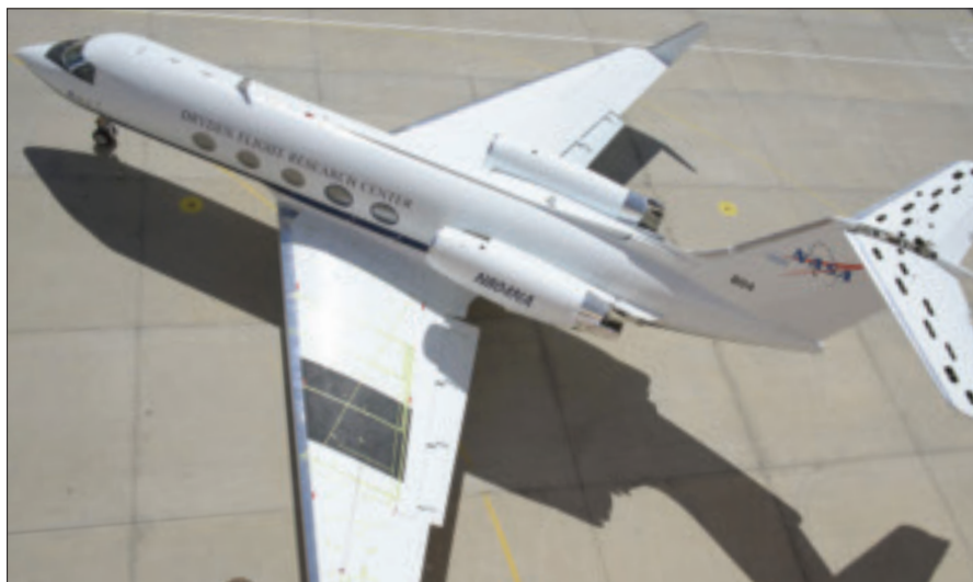
The area where the wing glove was placed on NASA Dryden's Gulfstream GIII is outlined in green. Image credit: NASA/Tony Landis.
