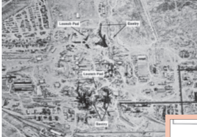
This HEXAGON panoramic image of the Area J facilities at Tyuratam was taken in August 1984. These two launch pads with their distinctive blast deflectors were part of Russia's buildup to send cosmonauts to the lunar surface competitively with Apollo. Four launch attempts between 1969 and 1972 failed. Courtesy NRO.
