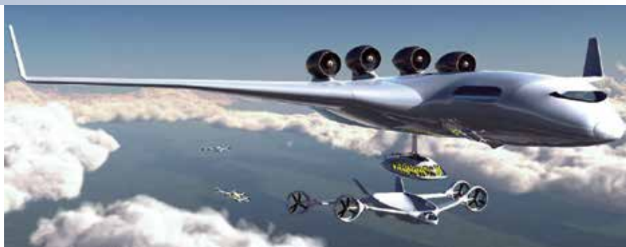
Simulations with existing planes could be a step toward a futuristic concept in which a giant passenger plane, called a cruiser, would pick up fuel and passengers from a smaller plane, called a feeder. Europe calls the project RECREATE, for Research on a Cruiser-Enabled Air Transport Environment.
