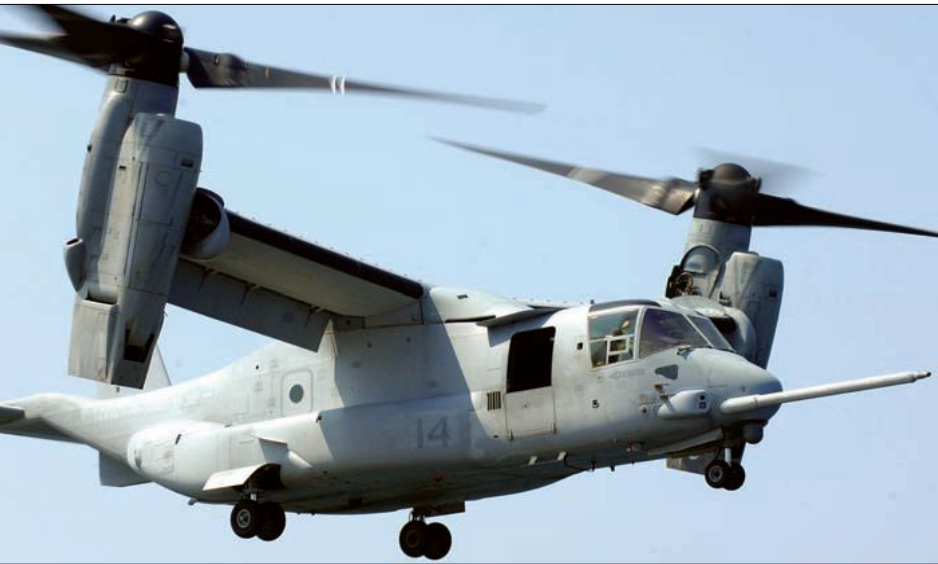
The V-22 Osprey tiltrotor provides the Marine Corps and Air Force with an aircraft that combines the vertical-lift characteristics of a helicopter with the superior range and speed of an airplane.
