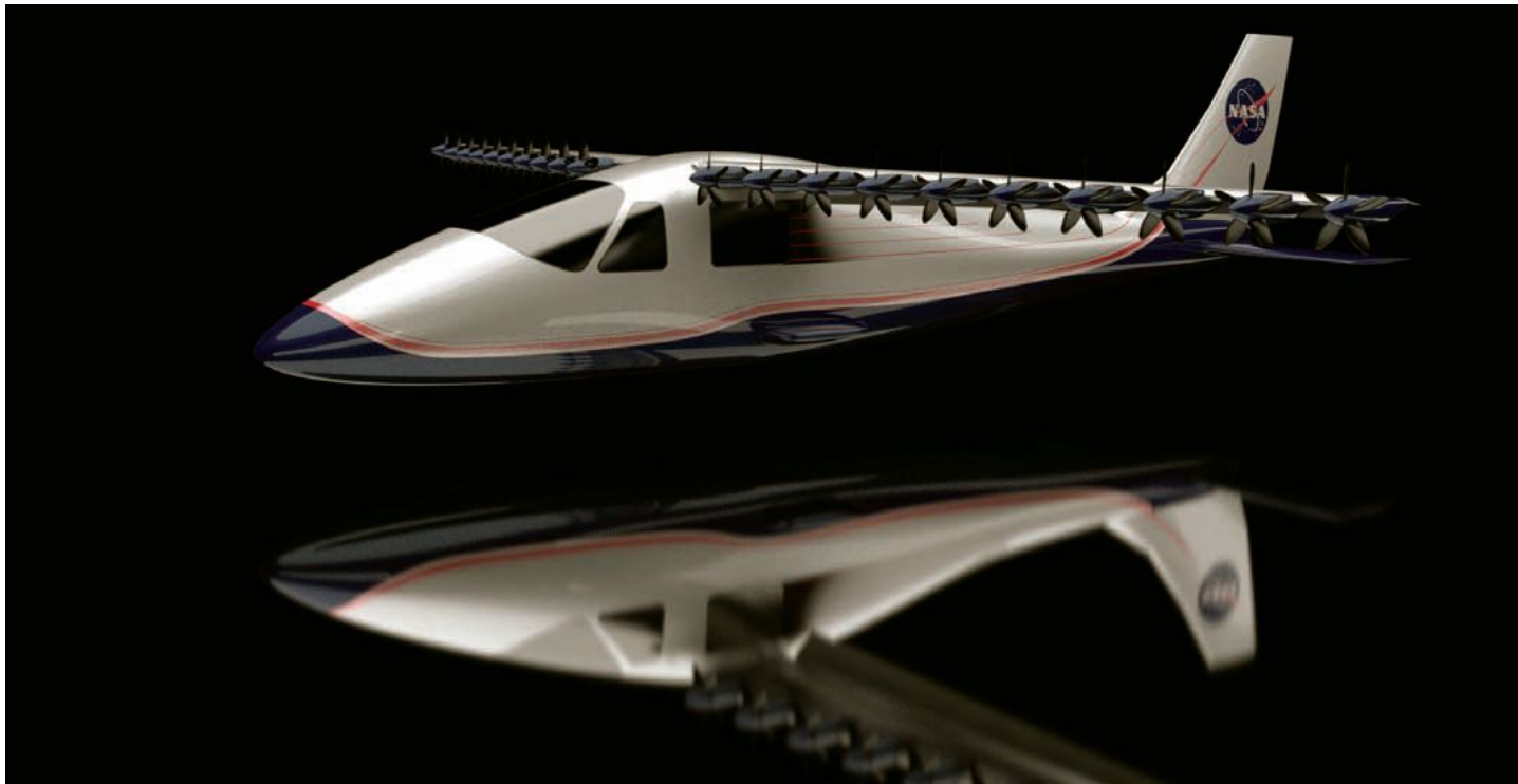
X-plane: A team led by NASA Langley Research Center plans to convert a conventional Tecnam plane into an electrically propelled experimental aircraft.
