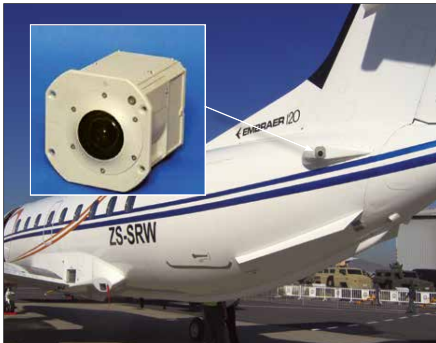
Saab's Civil Aircraft Missile Protection System autonomously detects incoming shoulder-launched anti-aircraft missiles and dispenses pyrophoric decoys to distract the threats.
