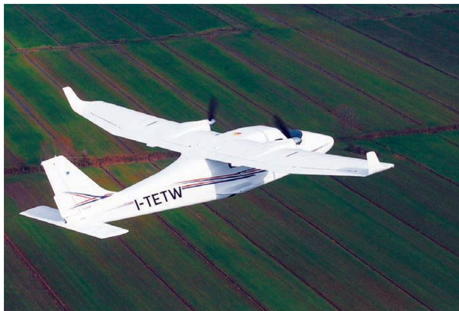
The conventional wings and engines of an Italian-built Tecnam P2006T air taxi will be replaced with composites wings and electrically-driven propellers.
