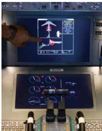
Commercial airline pilots steered a tanker aircraft and wide-body passenger aircraft in flight simulators to investigate aerial refueling of airliners.
