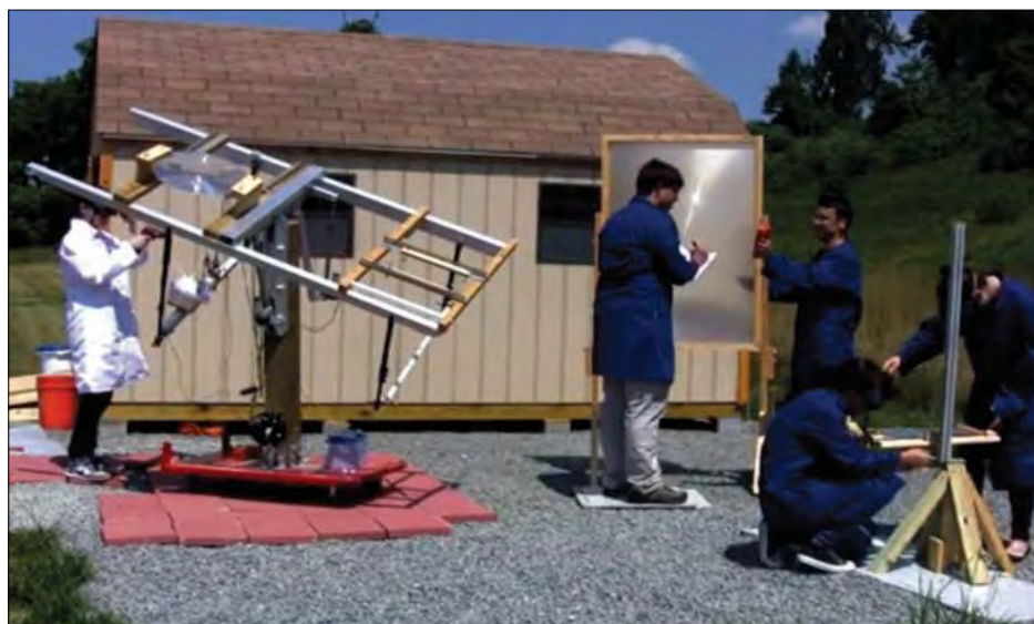
Researchers at George Washington University in Washington, D.C., used solar-generated electricity to convert carbon dioxide in the air to carbon nanofibers that could be used for aerospace parts.
