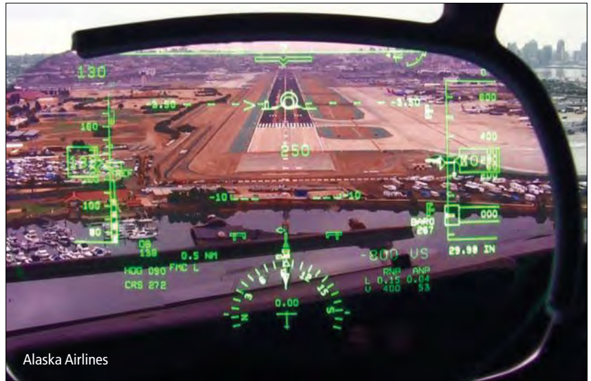
Alaska Airlines’ Heads-Up Guidance System projects flight information onto a glass screen as pilots approach San Diego. The Seattle-based carrier has pioneered the use of the guidance system to augment instrument landing systems to help with landings in fog and snow.
