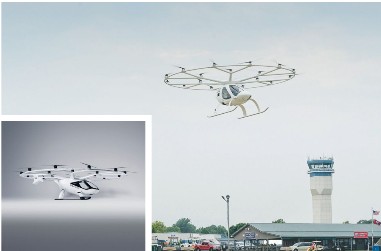
▲ A pilot flies the Volocopter 2X (top right) on a rehearsal flight before the EAA AirVenture in Oshkosh, Wis. The 2X is a prototype of the company's planned VoloCity electric vertical takeoff and landing aircraft (inset). Volocopter
