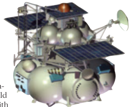
Flight elements of the Phobos sample return include the orbiter/lander that will orbit Mars and match orbits with Phobos until landing is possible. The drilling rig is at left. Atop that is the return vehicle that will fire back toward Earth carrying the descent module with soil and rock samples that will land in 2014.
