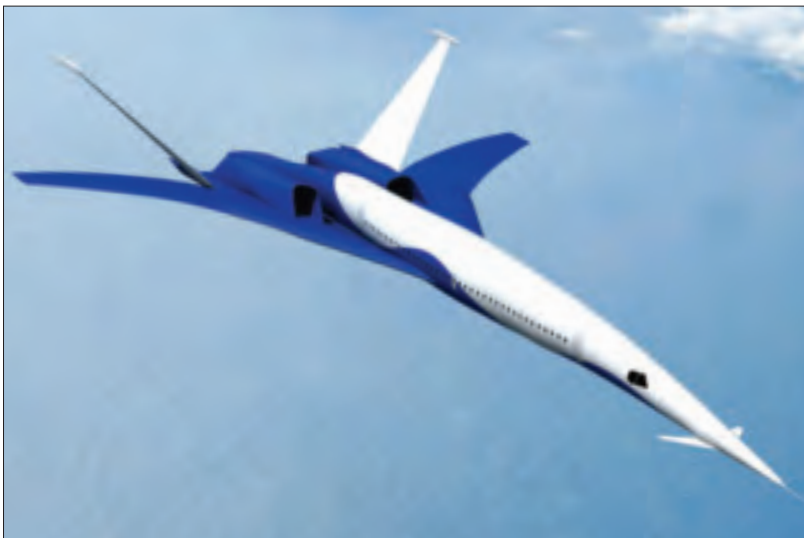
The Icon-II future aircraft design concept for supersonic flight over land comes from the team led by Boeing. A design that achieves fuel burn reduction and airport noise goals, it also achieves large reductions in sonic boom noise levels that will meet the target level required to make supersonic flight over land possible.
