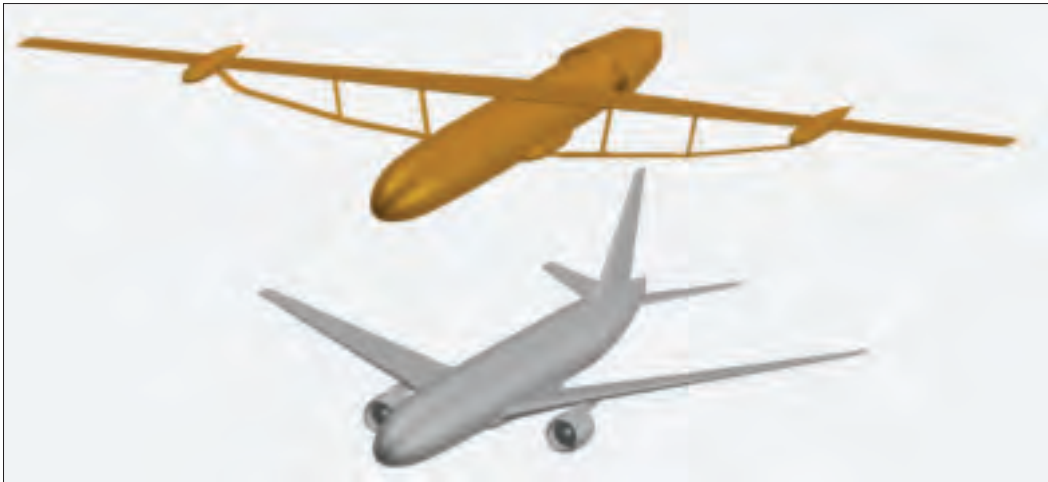
One truss-braced wing concept for a CTOL transport from VPI and Stanford University shows a longer wingspan than conventional aircraft.
