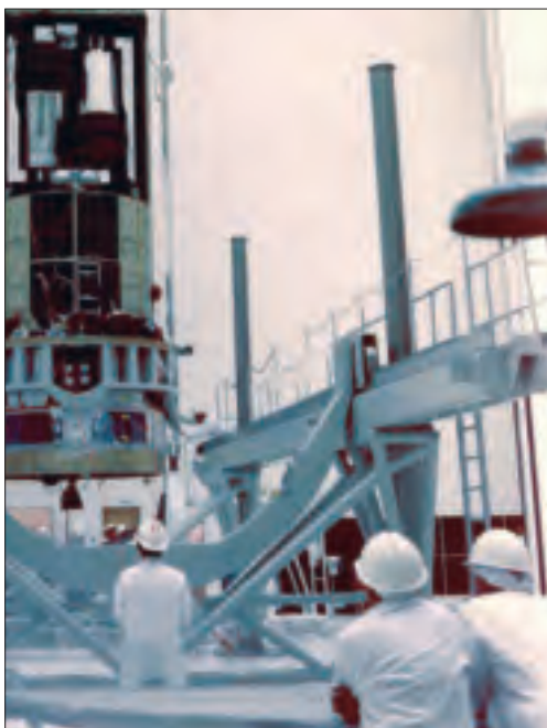
The HEXAGON system qualification vehicle is lowered into its 'A' frame by handling equipment during assembly at the Lockheed plant in Sunnyvale, California. Courtesy NRO.
