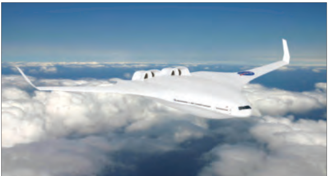
The hybrid wing body H-Series is from a research team led by MIT. It features embedded engines using variable-area nozzles with thrust vectoring, noise shielding, and advanced onboard vehicle health monitoring systems. Image credit: NASA/MIT/Aurora Flight Sciences.
