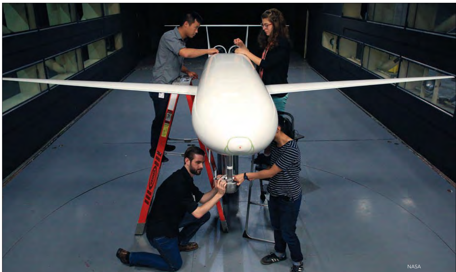
Shape of the future? MIT engineering students prepare the D8 airliner model for testing in NASA's 14-foot by 22-foot Subsonic Tunnel at the Langley Research Center in Virginia.
