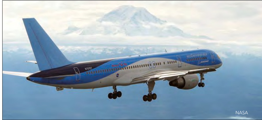
Drag reducer: In April, Boeing fitted the 757 ecoDemonstrator's tail with 31 air-blowing devices, part of an active flow control test to see if the tail can be made smaller to reduce drag without sacrificing control during takeoff and landing.
