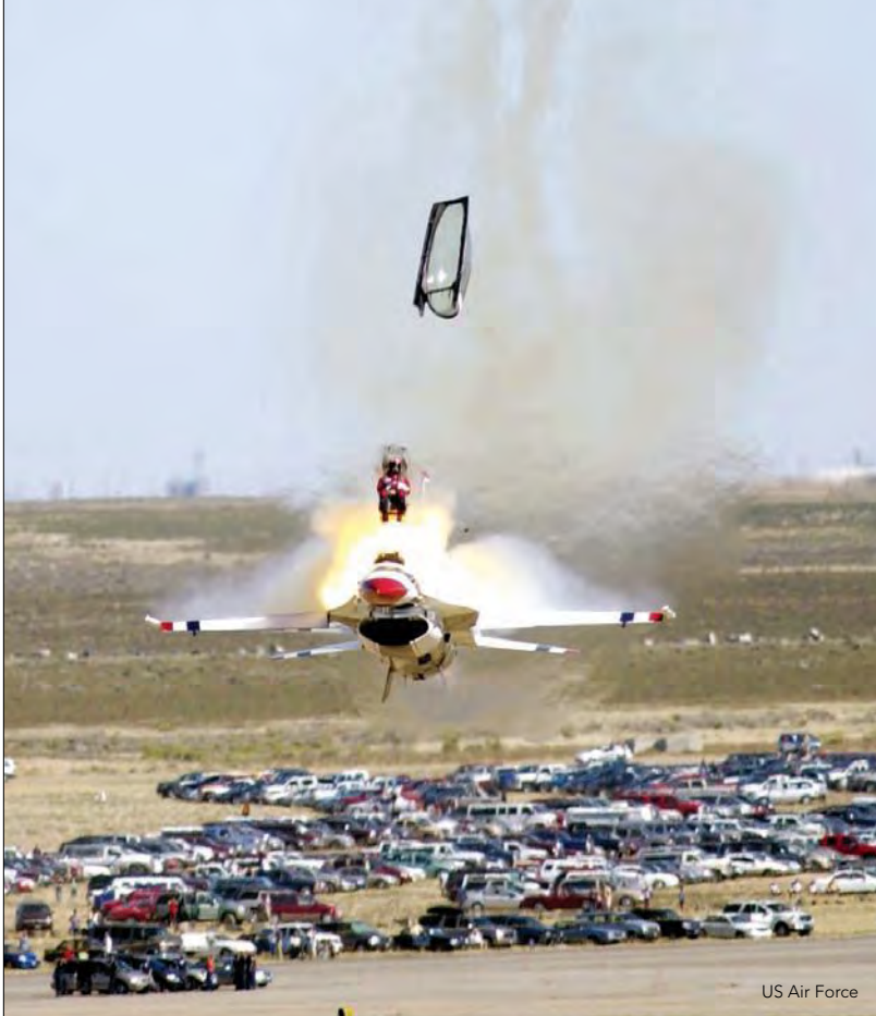
U.S. Air Force Capt. Christopher Stricklin uses an ACES 2 ejection seat to escape from his F-16 Thunderbird moments before it crashes at an Idaho air show in 1982. Stricklin, who steered the plane away from the crowd, was uninjured.
