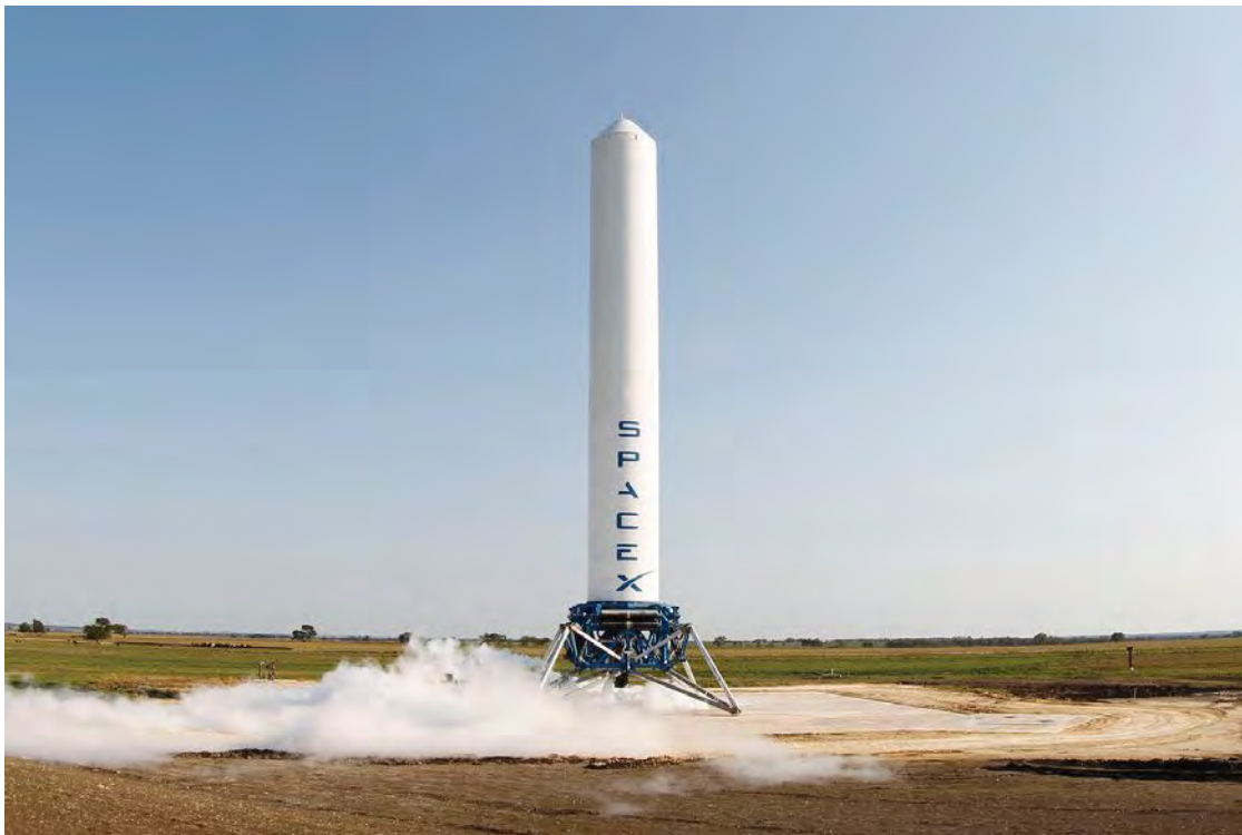
◀ SpaceX's Grasshopper vertical takeoff, vertical landing vehicle was a prototype reusable rocket that had eight test flights and landings in 2012-2013.
