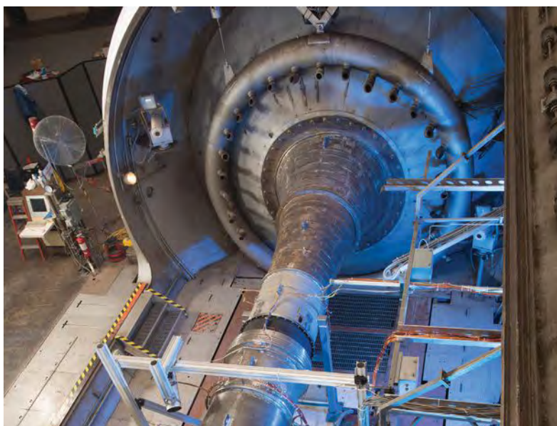
▲ This test cell at the Propulsion Systems Laboratory at NASA Glenn can create ice crystals like those at high altitudes.
