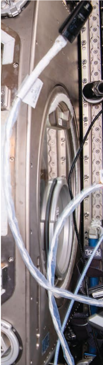
▲ This FOMS printer produced the company's first strands of ZBLAN aboard the ISS. NASA
