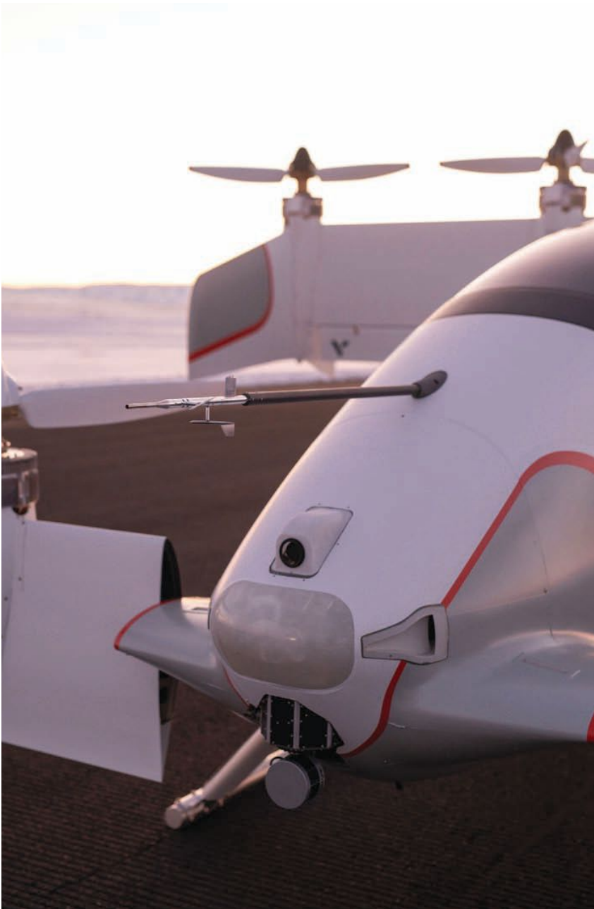
▲ The Vahana demonstrator, which took its last flight in November, had three types of sensors: cameras, lidar and radar. A 3 by Airbus
