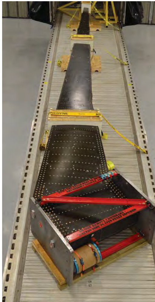
► Aurora Flight Sciences' 27 percent scale test article of the optimized tow-steered wingbox was tested in October at NASA's Armstrong Research Center in California.
