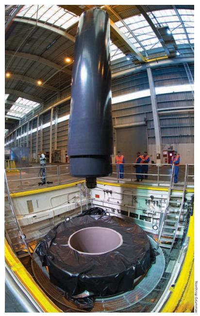
▲ A team of technicians removes the casting mandrel from a center segment after casting and curing the propellant.
