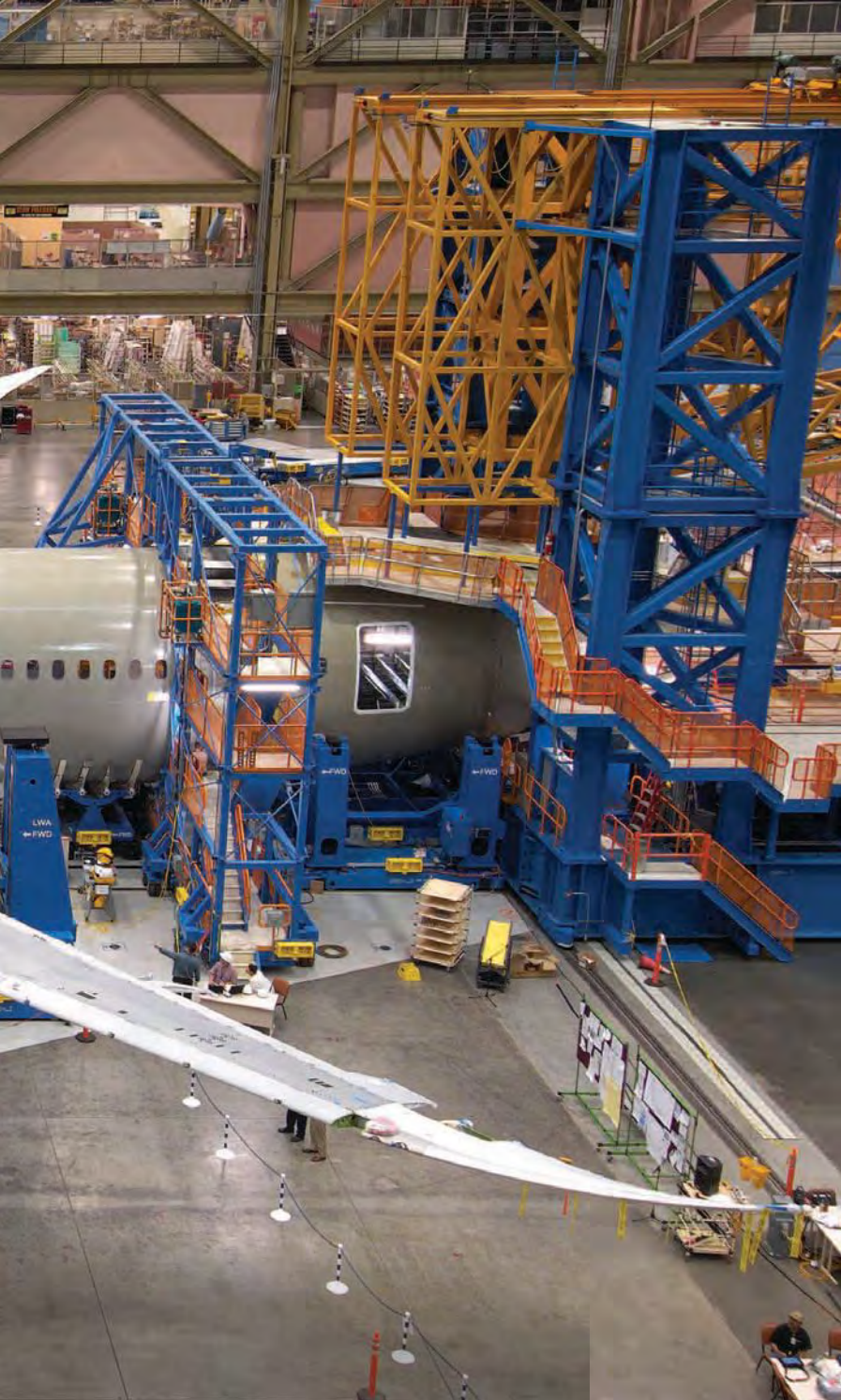
▲ A Boeing 787 on the assembly line in Everett, Wash.
