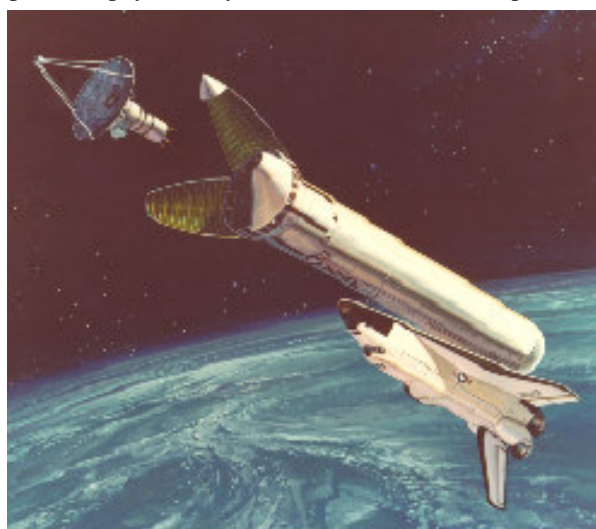
Figure 10. Large Diameter Low Density Payload Being Deployed From the Modified ET System. (Courtesy DARPA)
