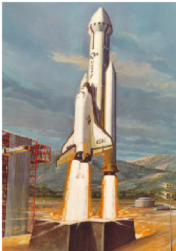
Figure 9. 10.6 Meter Diameter Hammerhead Configuration At Launch. (Courtesy DARPA)
