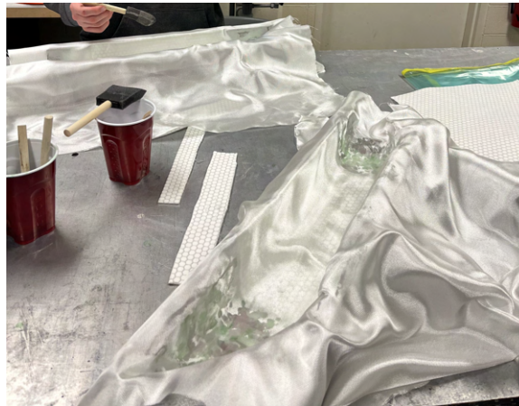
Figure 31: A second layer of fiberglass is placed over the Soric core during a fuselage layup
