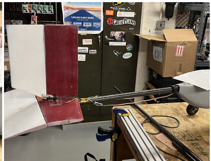
(b) Extended tail spar
