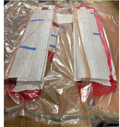
Figure 38: Wings Curing in the Vacuum Bag
