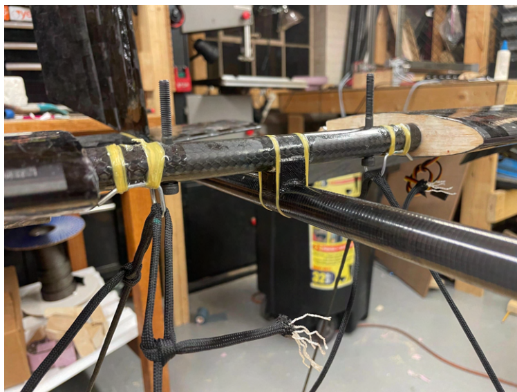
Figure 35: Aramid Lashing on Spar
