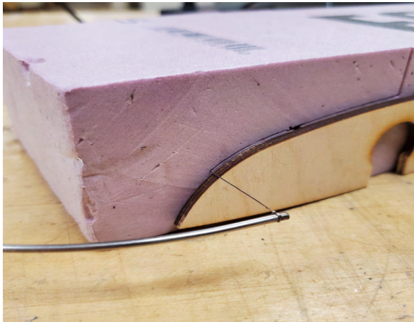
(a) Hot Wire Cutting by Hand Using a Plywood Stencil
