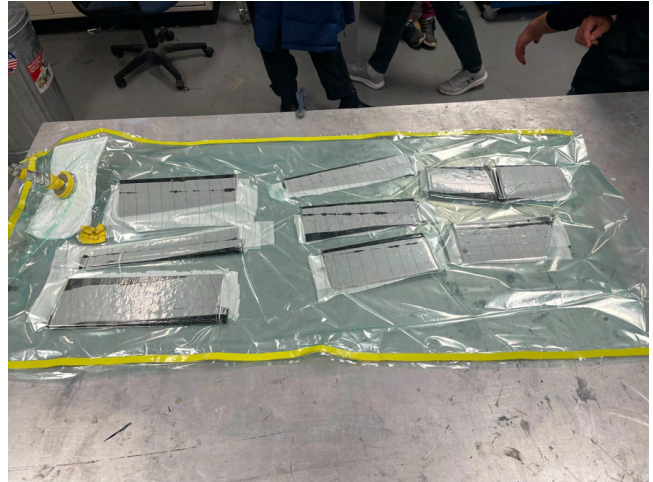
(b) Carbon Fiber Layup in Vacuum Bag
