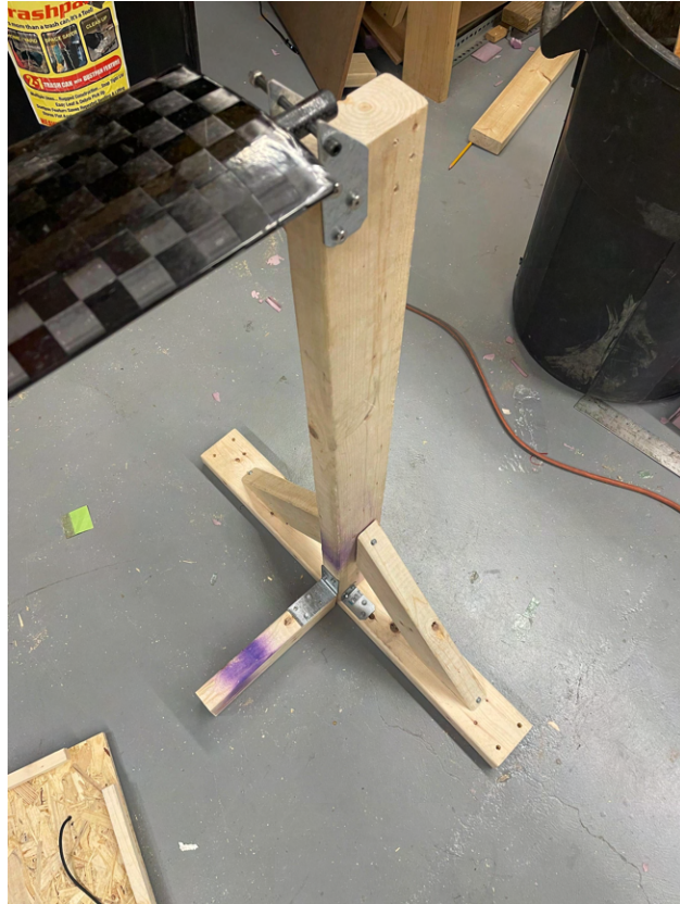
Figure 34: Load Test Fixture
