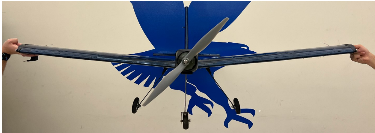
Figure 8-3: Weighted wingtip test
