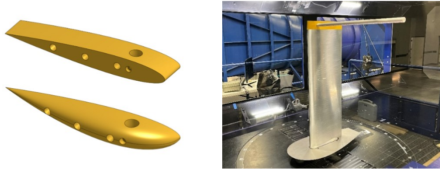
Figure 7-1: Blunt and blended wingtips (left) and 24-in JA with blunt wingtip in wind tunnel (right)
