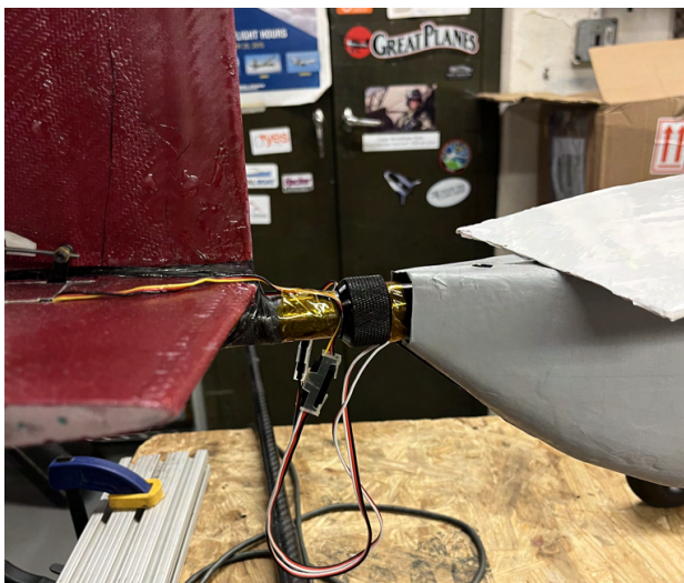
(a) Tail spar before extension
