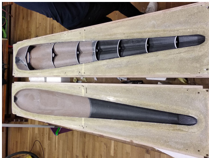
Figure 37: Building Composite Structure of the Fuselage Inside the Purenite Molds
