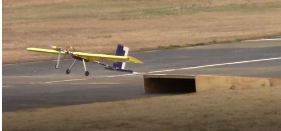
Figure 8.8. Ramp takeoff testing.
