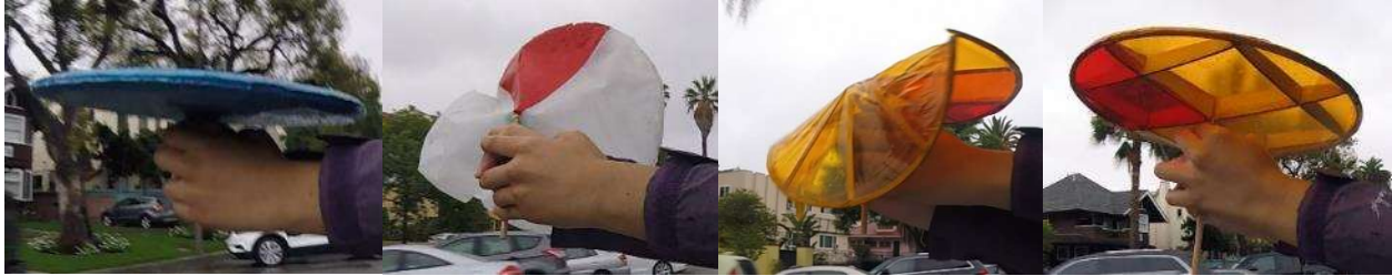
Figure 21: Radome testing with foam, fiber glass, radial plywood, and waffle plywood (left to right)
