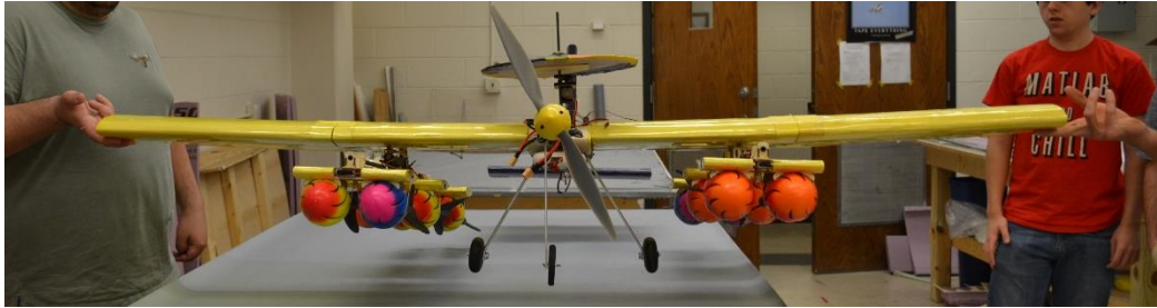
Figure 8.2. Wingtip test of fully loaded aircraft.
