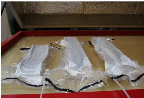
Figure 43: Vacuum bagging method for the skin
