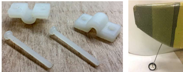
Figure 33: Nylon bolts and straps for nose gear (left) and fully integrated nose gear (right)
