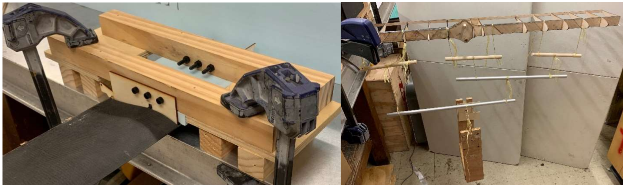
Figure 39: Wing to fixed fuselage mount (left) and whiffle tree loading on wing (right)
