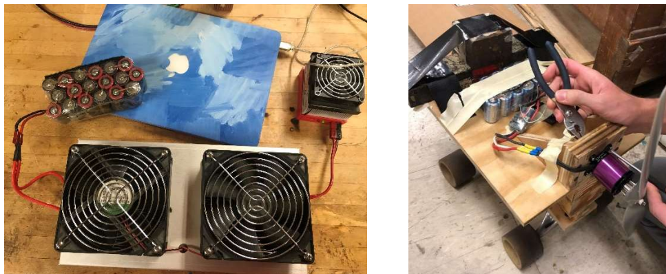
Figure 38: Battery Tester (left) and lab-built mule for propulsion system testing (right)
