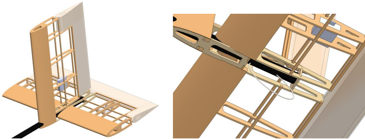
Figure 5.7. Empennage assembly (left) and the tail hook mounted to the bottom of the center line (right).
