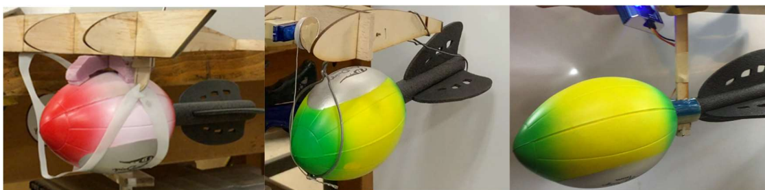
Figure 24: Attack store prototypes; Mylar strap, ring, and neck mechanisms (left to right)
