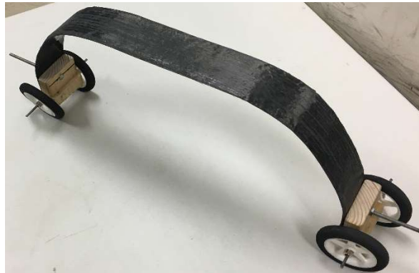
Figure 41: Bow gear used in static testing
