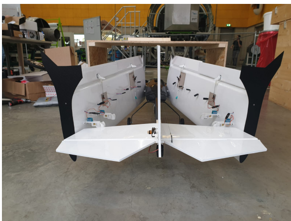
Figure 47: Roll through test with wooden box
