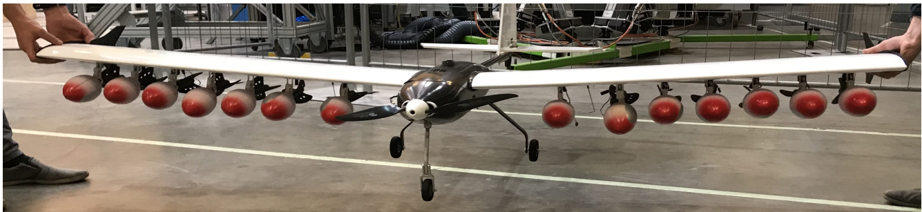
Figure 52: Wing tip loading test of the final design aircraft
