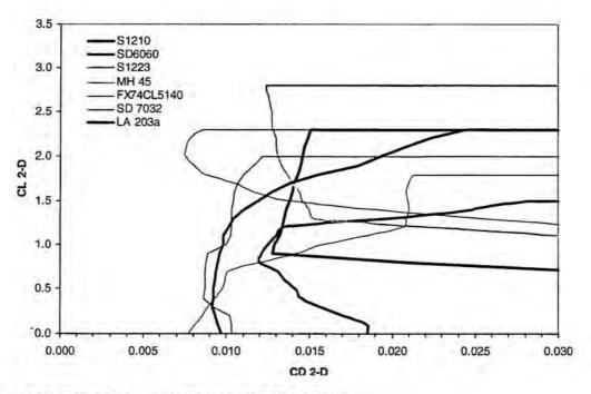
Figure 4.1 Airfoil drag polars, including geared flap effects.
