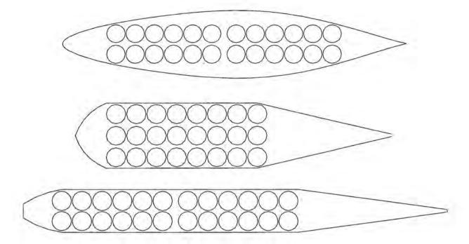
Figure 4.2 Fuselage payload configurations, 2 x 12 60% laminar, 3 x 8, and 2 x 12
