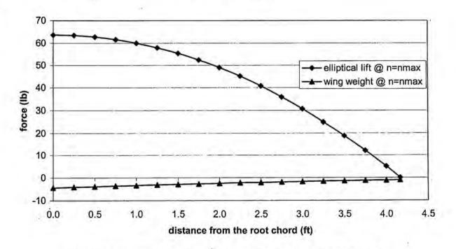
Figure 5.4 Flight load diagram due to lift and weight at load factor n=nmax
