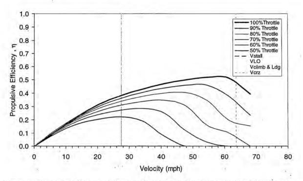
Figure 4.5 Propulsive efficiency plotted as a function of cruise velocity and variable throttle settings.
