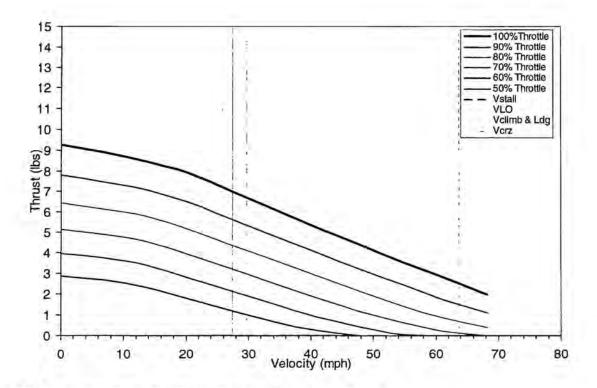
Figure 4.4 Affect of variable throttle and cruise velocity on thrust.
