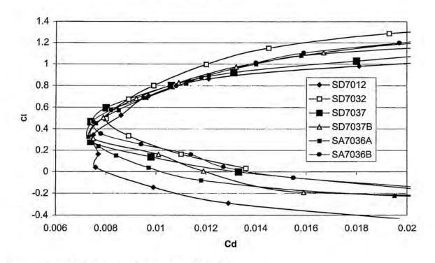
Figure 5.2 Airfoils evaluated for wing tip at Re=300K
