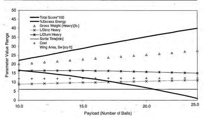
Figure 3.3. Payload capacity trade study results.
