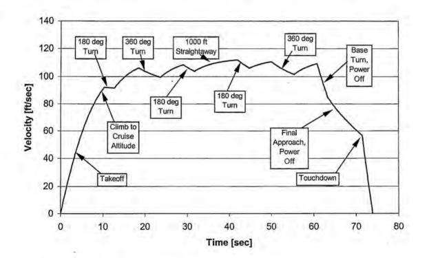
Figure 5.8 Velocity Profile during Position Mission Segment
