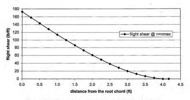
Figure 5.5 Flight shear diagram due to lift and weight at load factor n=nmax
