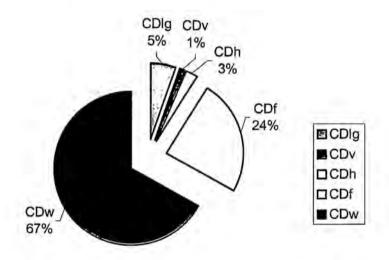
Figure 4.7 Drag breakdown at end of 3rd 180 deg for passenger delivery
