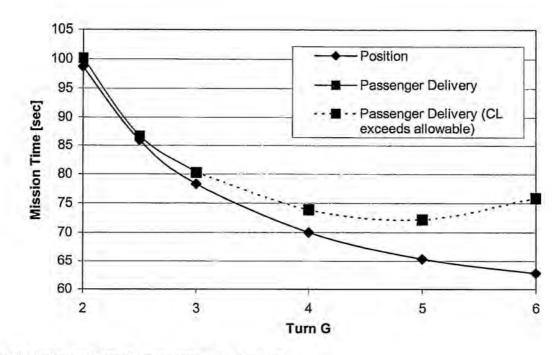
Figure 4.8 Limits on Turn G to reduce Mission Time
