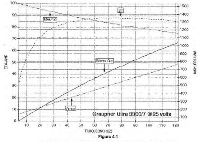
Initial testing on the Graupner Ultra 3300/7 motors showing vital statistics. Courtesy of Steve Neu
