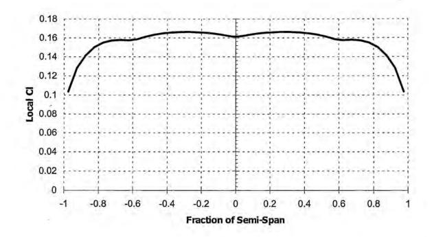
Figure 5.1 Span wise CI distribution for final wing planform
