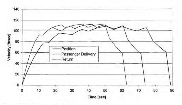
Figure 5.9 Velocity Profiles for all mission segments
