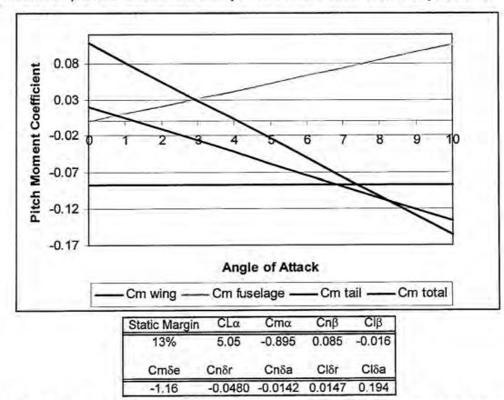
Figure 14: Coefficient of Moment of Aircraft Components Versus Angle of Attack and Stability Derivatives
