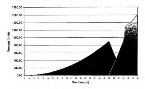
Figure 4.2.12 Shear Loading for semi-span of wing spar in 10G unloaded turn. Red denotes outer wing section, and blue denotes center wing section.
