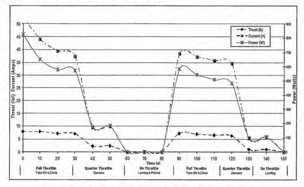
Figure 5.1: Simulated Mission Profile with Thrust, Current, and Power
