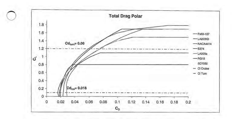
Figure 4.2.2 Graph of C<sub>L</sub> v C<sub>D</sub> for various airfoils. Dashed lines denote drag coefficients at cruise and turning conditions for the airfoil chosen (Fx63-137)
