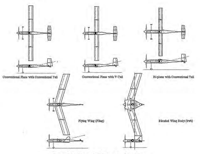
Figure 3.2.1 Conceptual design configurations
