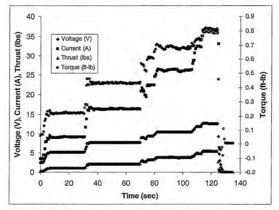
Figure 4.2.7 Time trace of data for Graupner 3300-06 using a power supply and a Bolly carbon 24 x 24 prop
