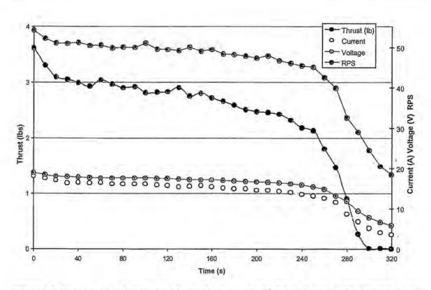
Figure 4.8: Motor/Battery Performance Curve for Graupner 3300-6, 20" Prop., 1.72 gear ratio, and 16 CP 1300 Cells at Half Throttle.
