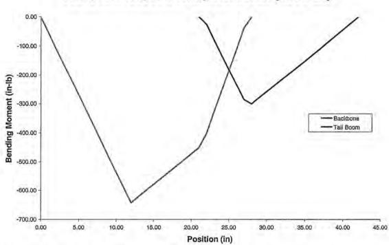
Bending Moment Diagram for Fuselage Structures during hard landing
