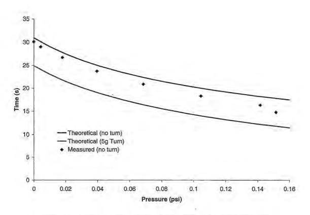
Figure 7.1.5 Theoretical vs. Measured drop times for different pressures.
