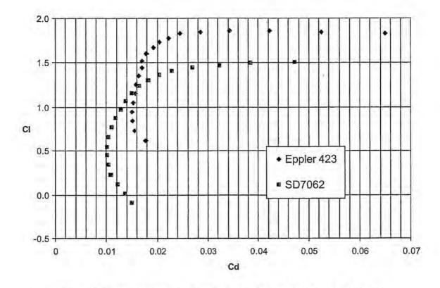
Figure 4.2: Drag Polar and Lift Curve for SD7062 and E423 at a Re of 250,000
