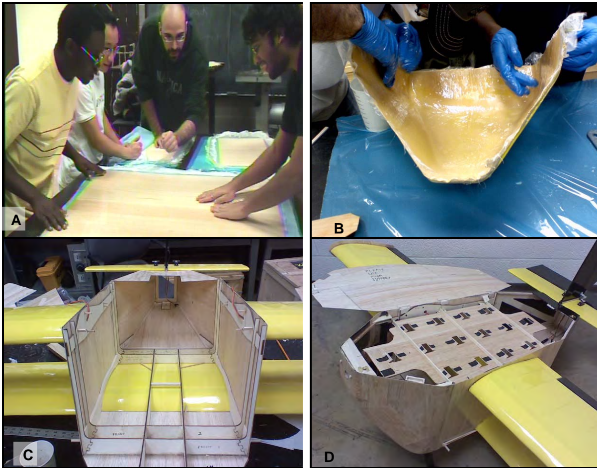
Figure 6.1—(a) Laminate Sheets, (b) Nose Lay-up, (c) Fuselage Structure, and (d) Final Fuselage
