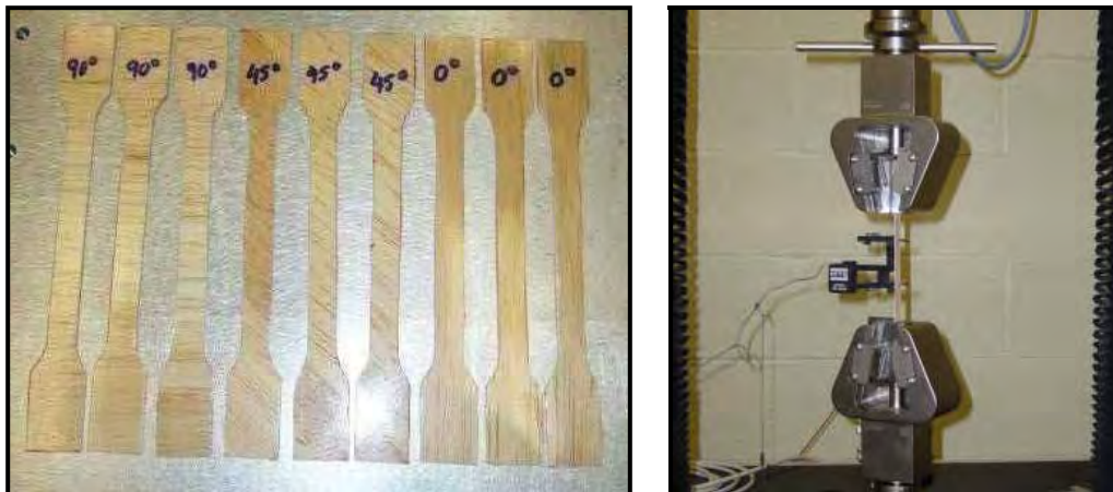
Figure 7.3 – (a) Prepared Specimens and (b) Testing in Progress
