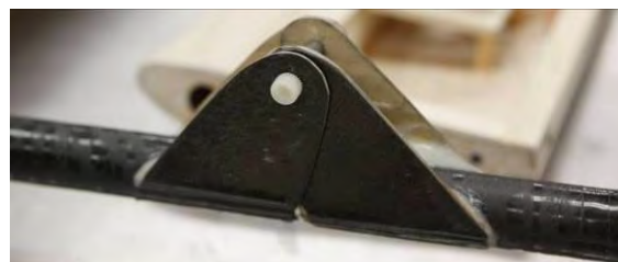
Figure 41: Carbon fiber fuselage tube and tail boom hinge.
