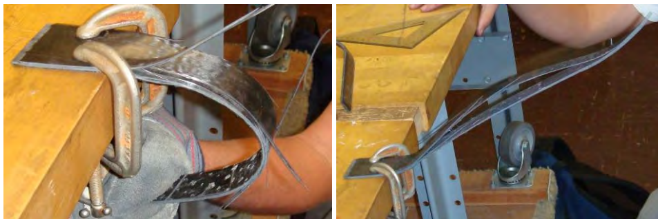
Figure 47: A half bow main gear (left) was loaded past its predicted maximum before delaminating (right).
