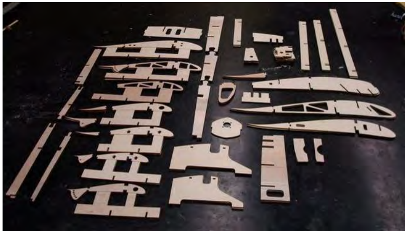
Figure 6.4 – CAD developed, Laser Cut Structural Elements and Tooling
