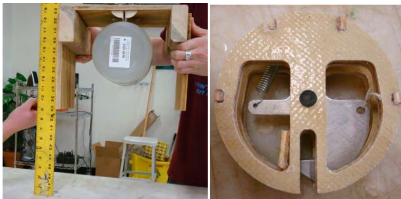
Figure 53: Centerline Payload Release Mechanism Testing
