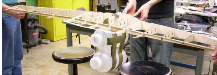
Figure 7.6– Ground Mission Wingtip Test
