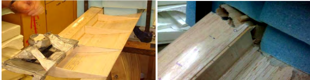
Figure 46: A hybrid wing section's (left) spar and D-box ruptured at maximum load (right).
