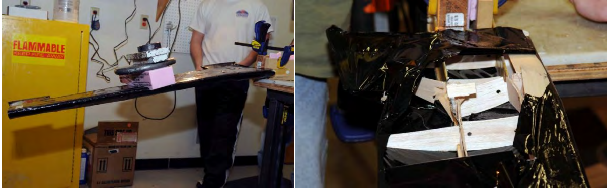
Figure 8.2 — (a) Full Wing Cantilever Test; (b) Subsequent Failure of the Wing
