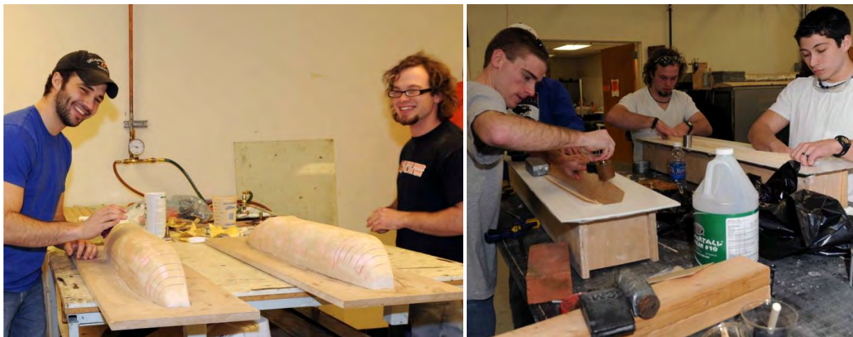
Figure 6.3 — (a) Fabrication of Fuselage Molds; (b) Fuselage Skin Lay-Up in Molds
