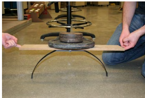
Figure 7.3: Landing Gear Under 3 G Simulated Load
