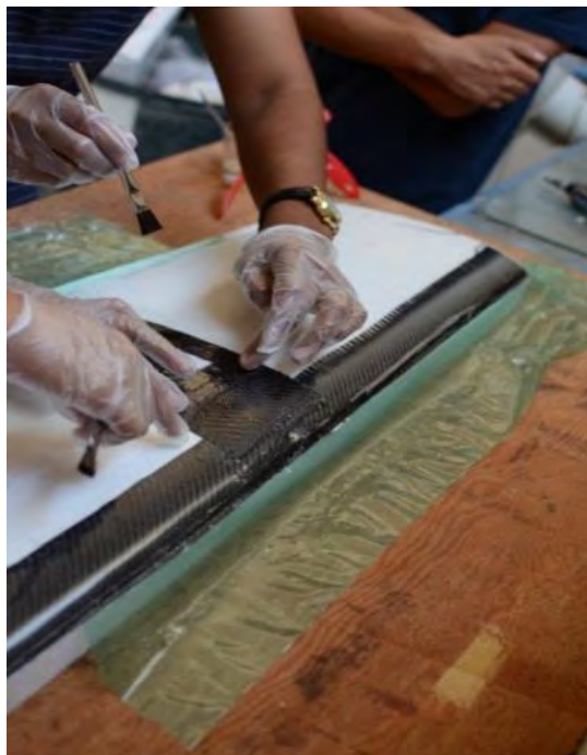
Figure 53 – Carbon Fiber Layup of the SD7032 Airfoil
