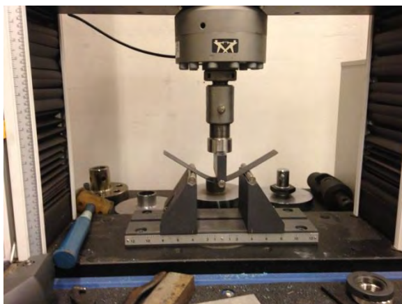
Figure 63 – Three Point Bend Test for Carbon Fiber (left) XPS Foam (right)
