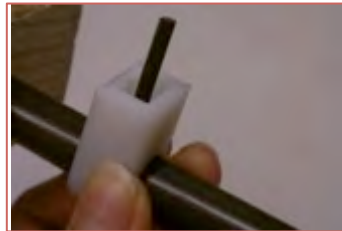
Figure 8.6 Screw attachment failure
