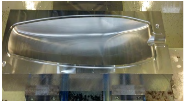
Figure 54 – Platen Press Machine (left) Bladder Mold (right) of Fuselage
