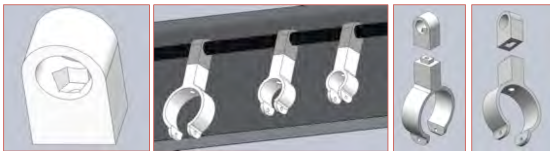
Figure 5.17 External store attachment design
