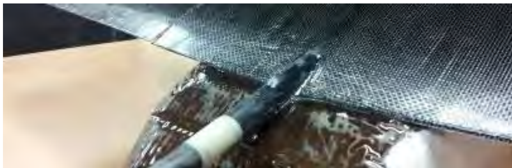
Figure 55 – Spar Connecting Empennage to Bottom Wing Using Carbon Fiber Strip Secured With Epoxy
