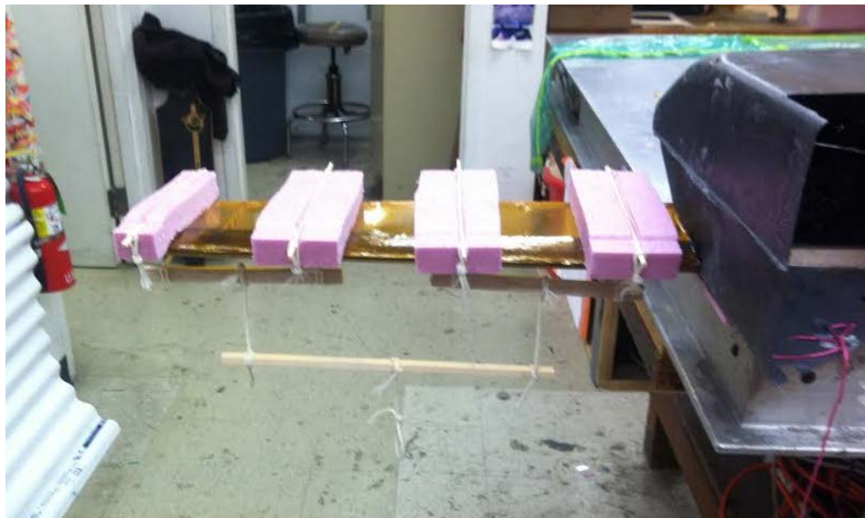
Figure 31: Static load testing of wing in whiffle tree tool, mounted upside-down to carbon nose.
