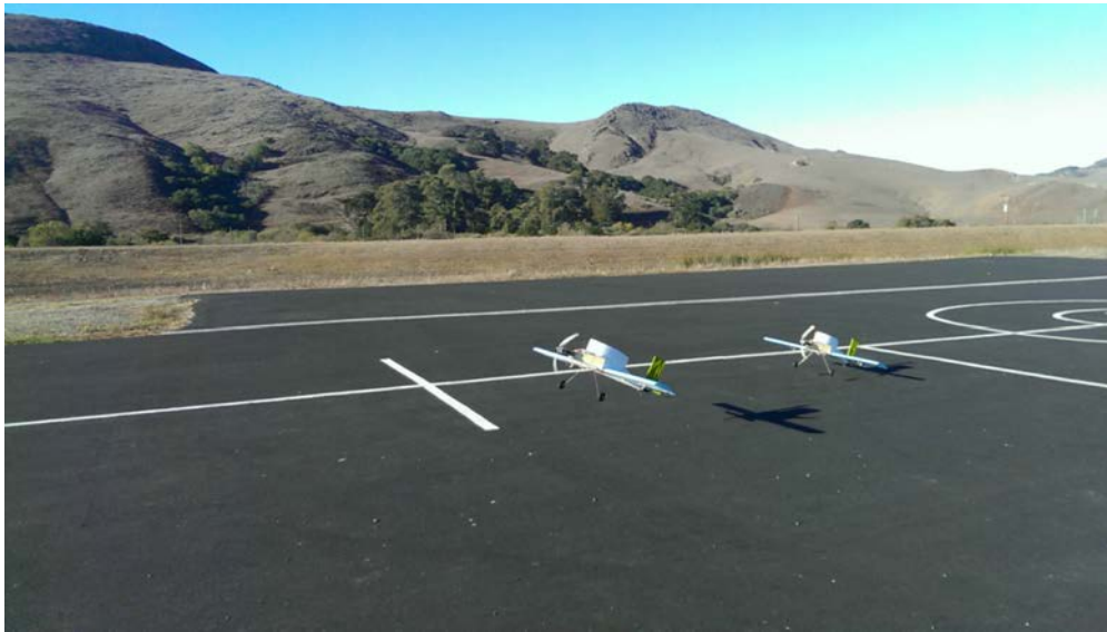
Figure 7.2 Foam Prototype Meeting Takeoff Distance Fully Loaded
