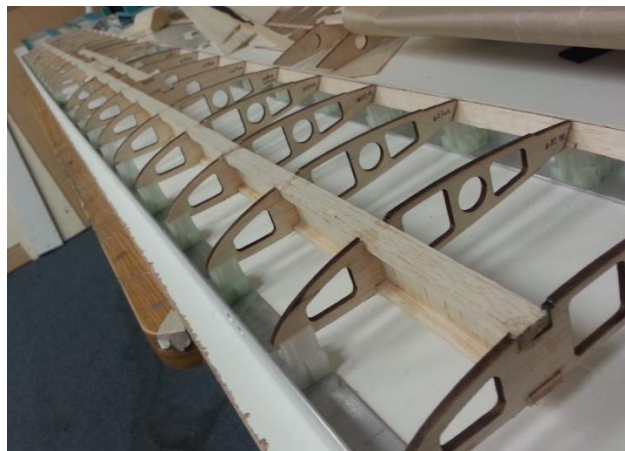
Figure 6.1: Balsa Built up Assembly
