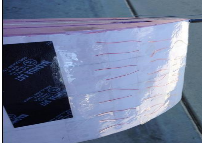
Figure 7-2: Flow Test with Flow Visualization Tufts Attached Aft of the Fuselage
