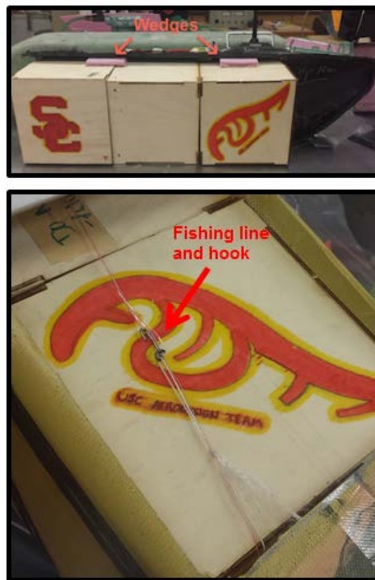
Figure 10: Foam wedges (top) and fishing line and hook mechanism (bottom) tested for Mission 2 payloads.
