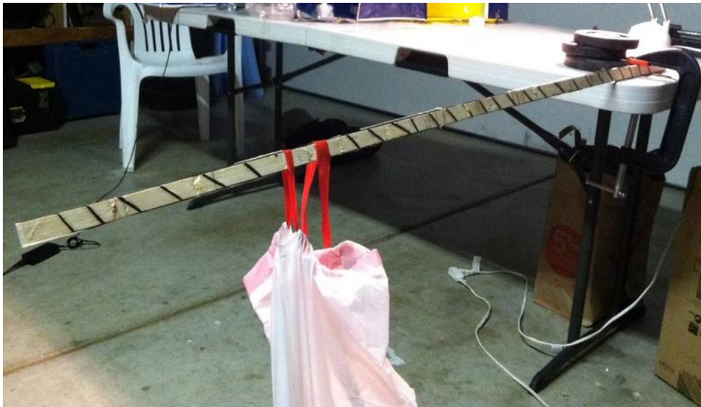
Figure 7-1: Strength Test Performed on the Spar
