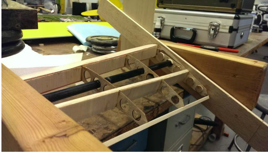
Figure 7.5 Failed Wing Section During Torsional Testing
