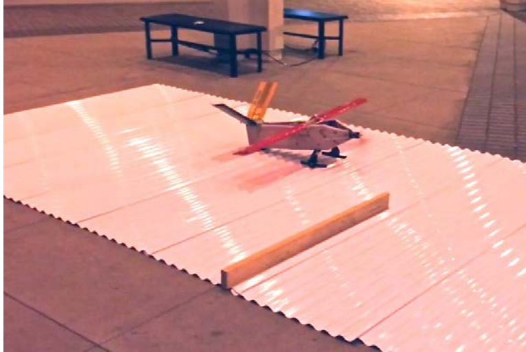
Figure 30: An airplane with prototype landing gear maneuvering around obstacles in the Taxi Mission simulation.
