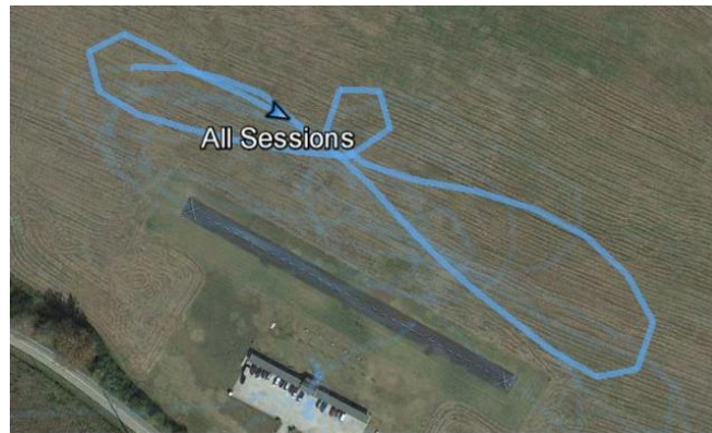
Figure 8.6: Trajectory of aircraft during competition laps from GPS data.
