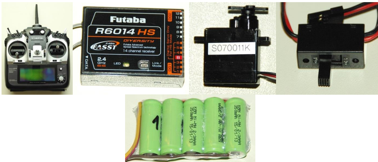
Figure 5.7.: Transmitter, receiver, servo motor, switch and receiver battery pack
