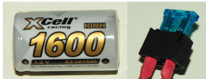
Figure 5.5: XCell racing 1600 NiMh cell and blade type fuse in socket
