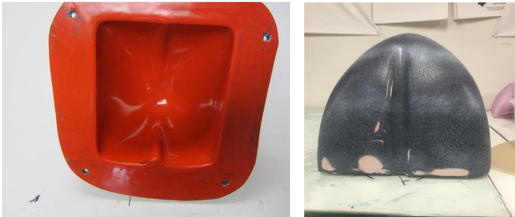
Figure 6.2: Front Fairing Molds
