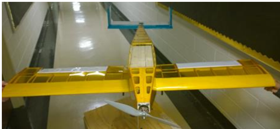
Figure 8.4: Wingtip Structural Test with Full Payload.
