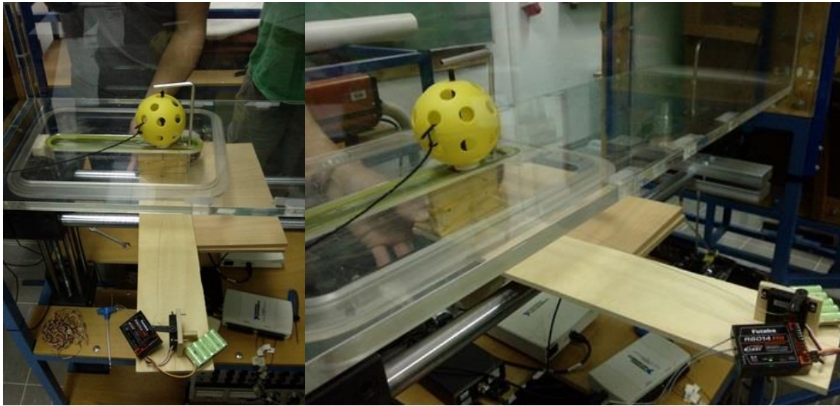
Figure 7.3: Testing of ball drop mechanism in wind tunnel
