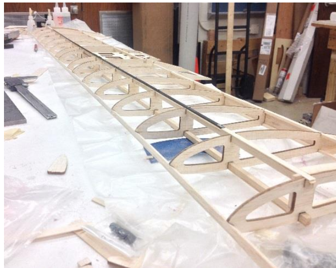
Figure 6.1: Prototype aircraft wing in production.
