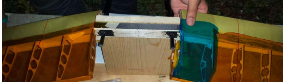
Figure 8. 1: Wing test failure
