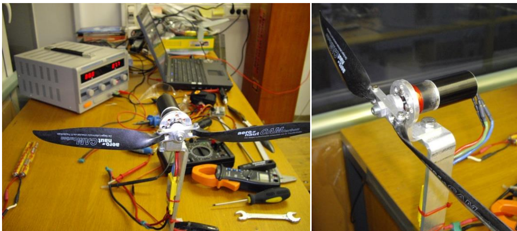
Figure 7.1: Propeller static thrust test
