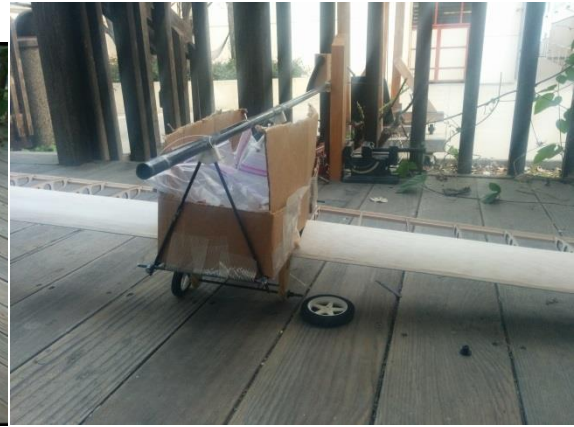
Figure 7.2: Landing gear test failure
