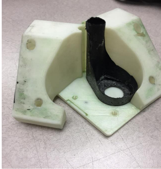
Figure 6.6: Motor Mount and 3D Printed Mold
