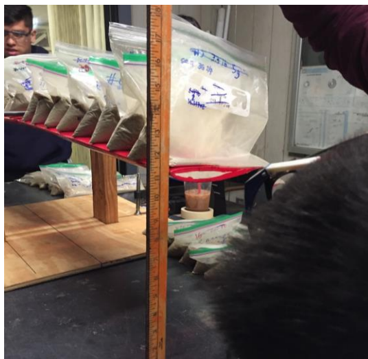
Figure 8: 2 Measuring leading edge deflection during wing bending testing.
