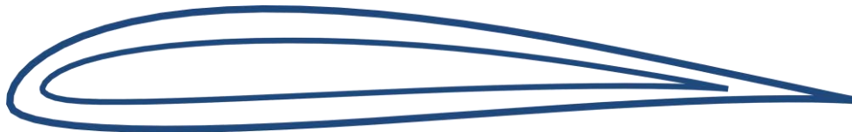
Figure 4.6: S4110 inside of SD7062 airfoil.
