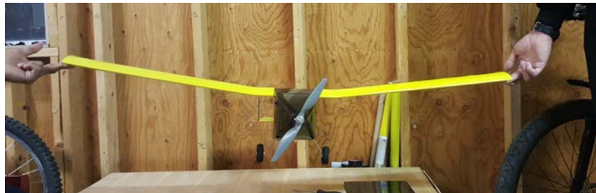
Figure 7.1.2: Wing tip test of PR Aircraft w/ payload (Simulating +2g acceleration)
