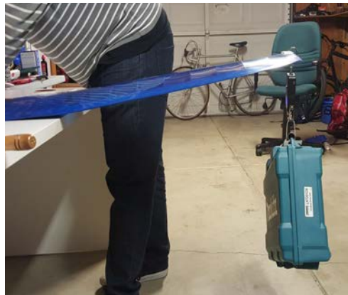
Figure 7.1.1: Stress testing first complete wing structure.
