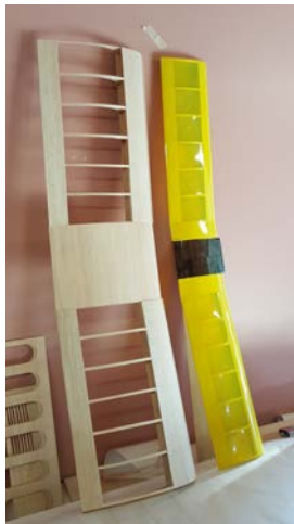
Figure 5.2.2: MS wing under construction alongside completed PR wing
