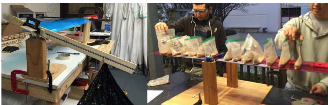
Figure 7: 2 Wing Torsion Testing and Wing Bending Testing
