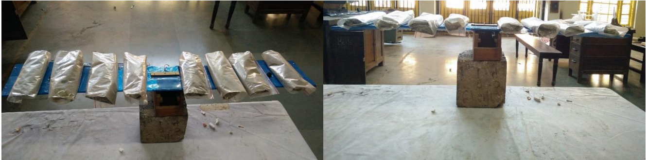
Figure 7.2.1 (a): Wing loading test
