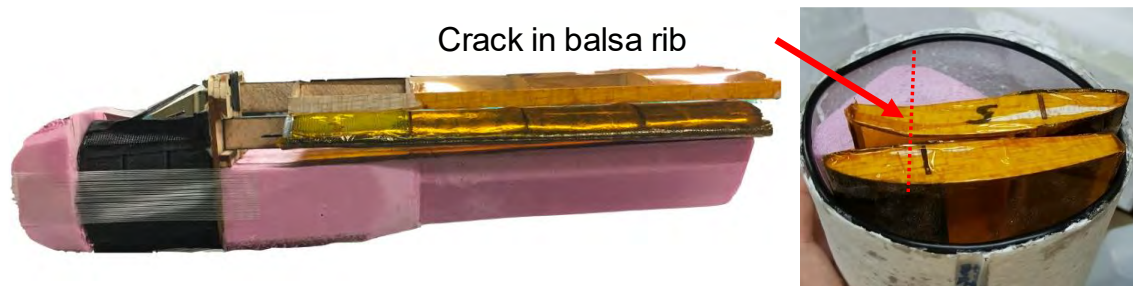
Figure 43: Drop test mule, simulating weight of the aircraft on balsa wings. The failure in the balsa ribs resulting from the worst case loading led to improved load transfer in the balsa wings.
