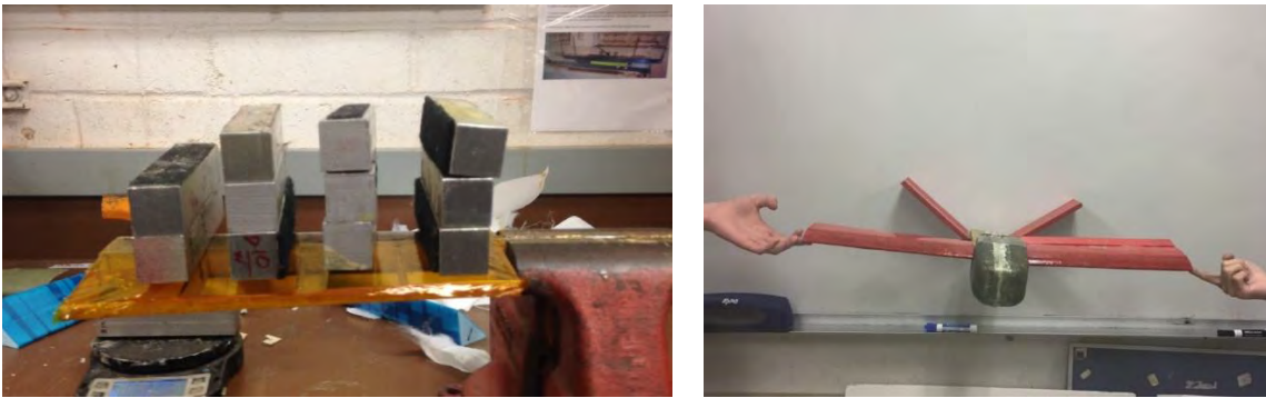
Figure 37: Setup for elliptical flight load testing (left) and wingtip testing (right).
