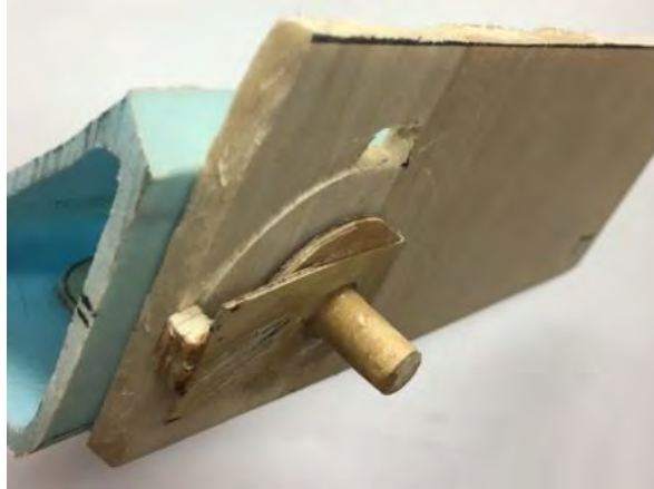
Figure 23: Preliminary design mockup of the empennage and locking mechanism.
