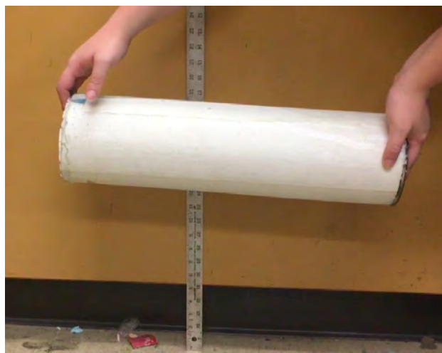
Figure 38: Drop testing was conducted with the fully loaded aircraft stowed inside the launch tube.
