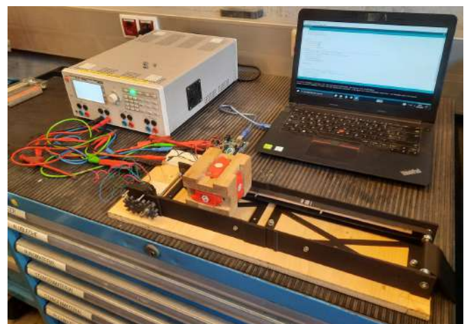
Figure 50: Deployment mechanism test set up
