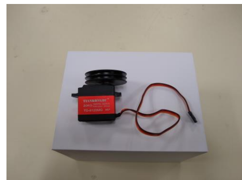
Figure 6.1: Pulley Servo with Dual Spool
