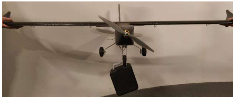
Figure 54: Wing tip loading test of the final design aircraft
