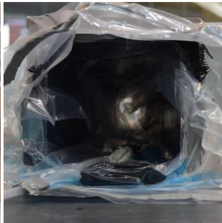
Figure 42: Cowling vacuum bagging
