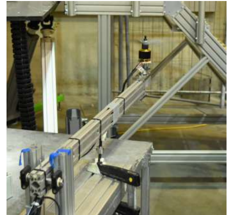
Figure 49: Static thrust test set up
