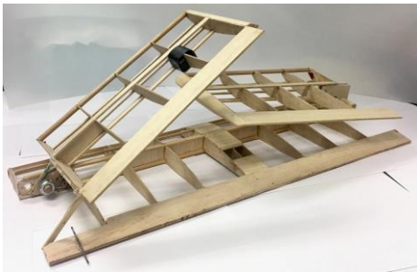
Figure 7: Wing Folding Mechanism
