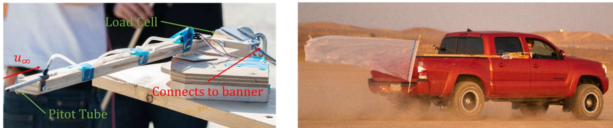
Figure 36: Banner test setup. The testing rig is shown on the left, and a representative data run is shown on the right. The rig was mounted one truck width away to be isolated from the truck wake.
