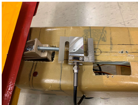
Figure 38: Strain gauge mounted on the test aircraft for banner flight tests.
