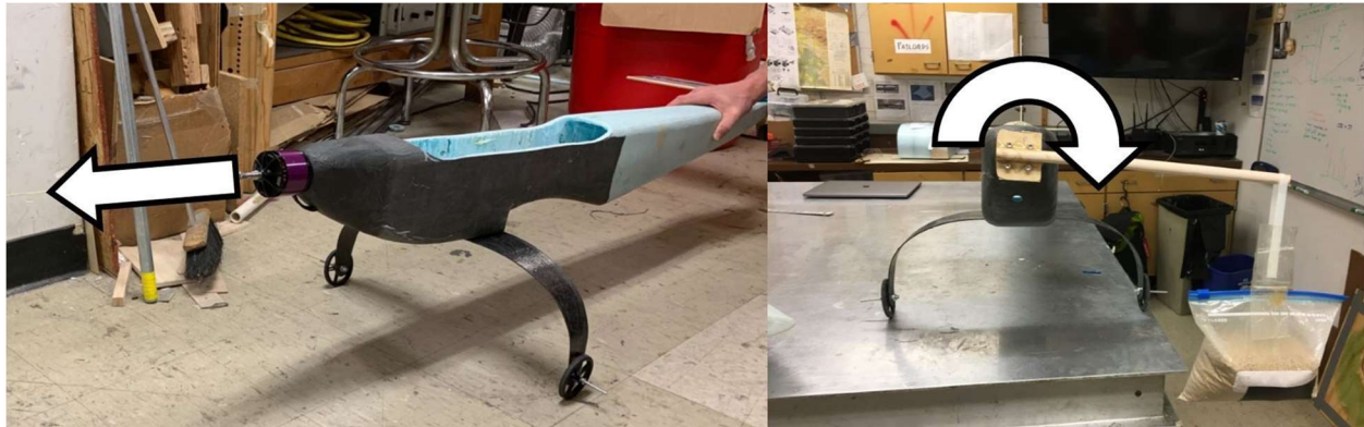
Figure 41: Simulated testing of motor thrust (left) and torque (right).
