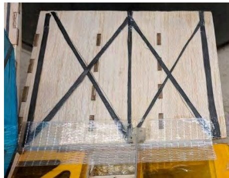
Figure 5.4: Elevon attachment mechanism
