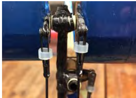
Figure 37. Lashed Bushing and Tail Boom
