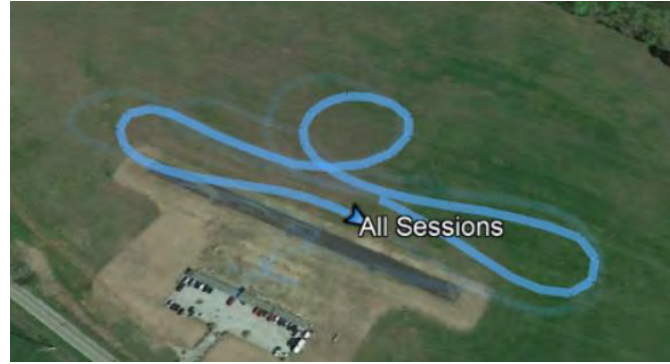
Figure 8.4: Trajectory of aircraft during competition laps from GPS data
