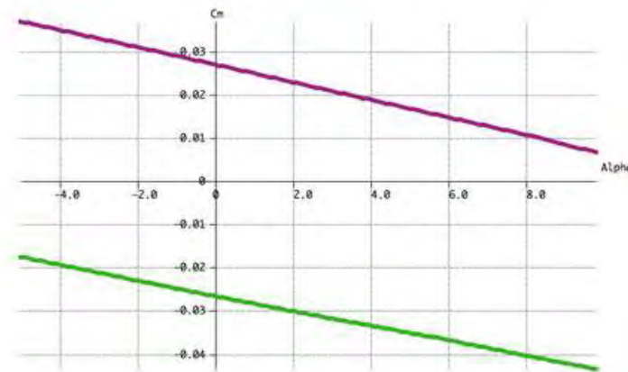
Figure 13 - C_M vs Angle of Attack
