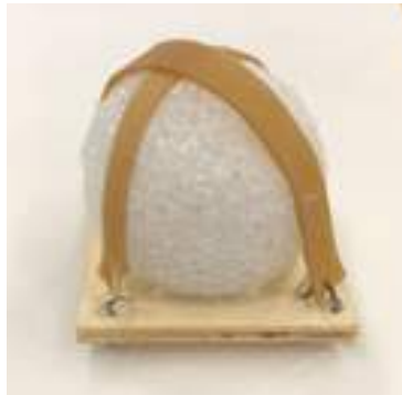
Figure 17 - Passenger Restraint System with Largest Passenger Installed
