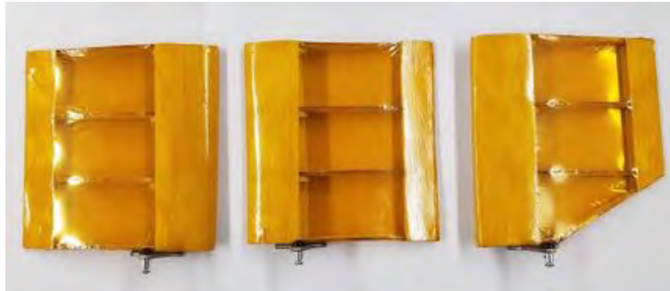
Figure 35. Lightweight, Removable Control Surfaces
