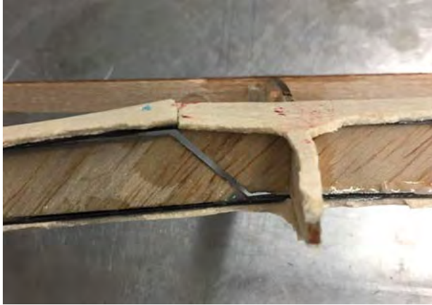
Figure 44: Shear web failure at integration point
