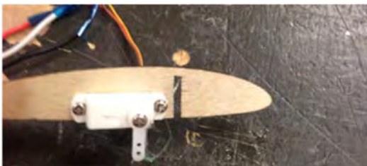
Figure 31: Wing servo LRU
