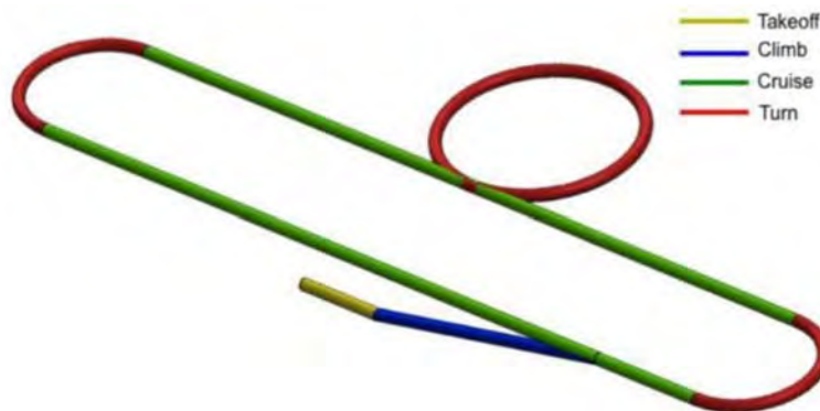
Figure 9: Flight model used in PlaneTools, indicating all phases of flight.
