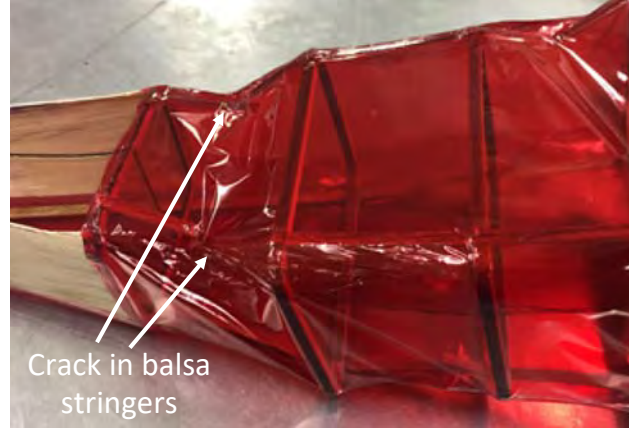
Figure 45: Fuselage failure in tail arm
