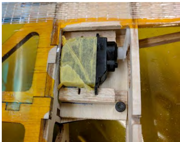
Figure 5.6: Removable servo prototype
