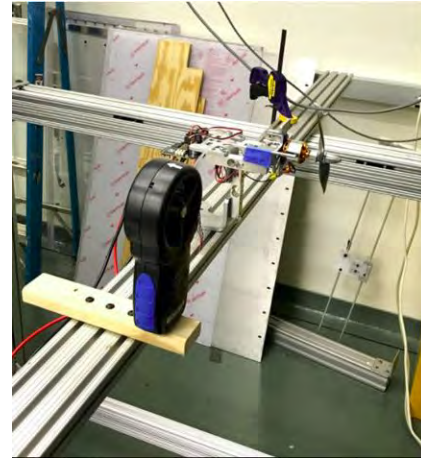
Figure 41. RCbenchmark Series 1580 Specification and Test Stand
