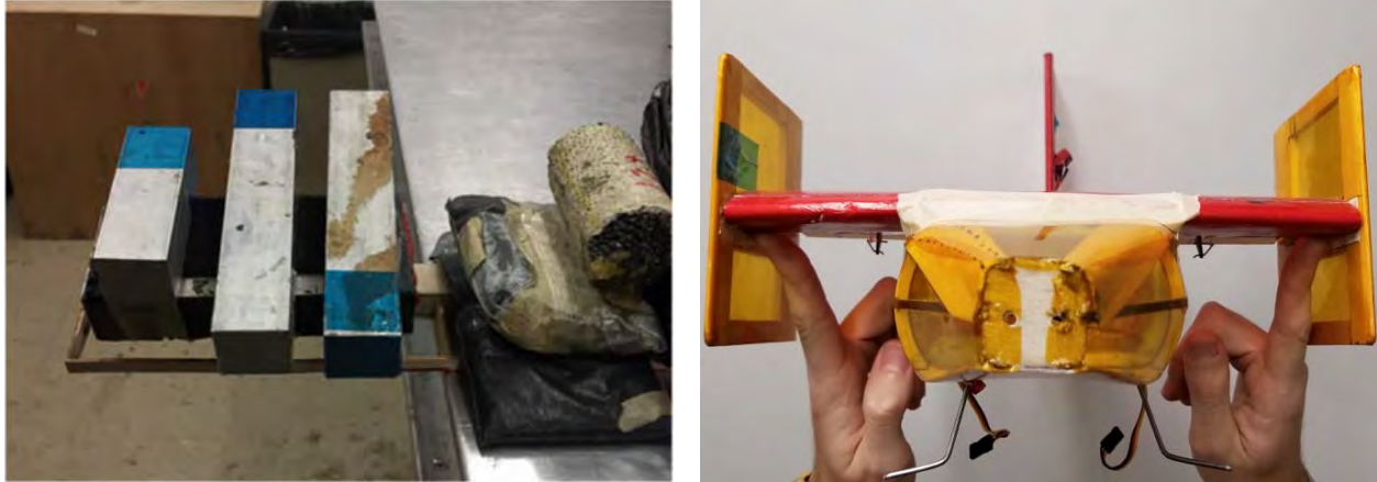
Figure 38: Setup for load testing with ballast blocks (left) and wingtip testing (right)
